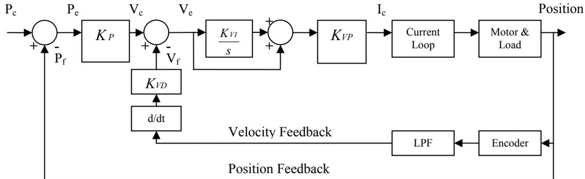
**Figure 5.** A simplified block diagram of cascaded position-velocity loops.
