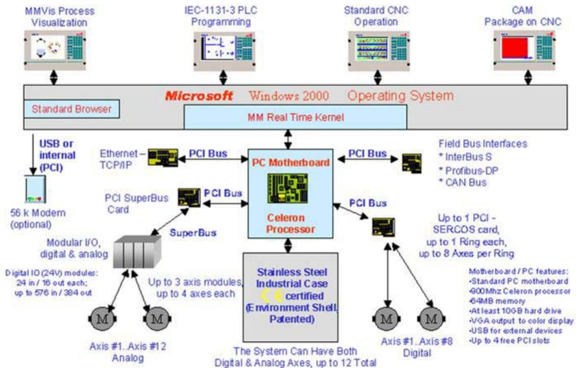
Figure 4. PC-Based CNC Architecture (MachineMate® PC-Based CNC Controls)
