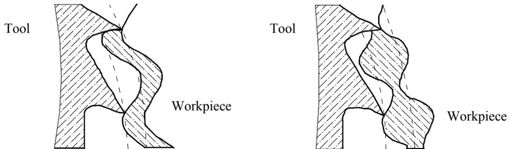
Figure 8 – Chip thickness variation for stable (left) and unstable (right) conditions
