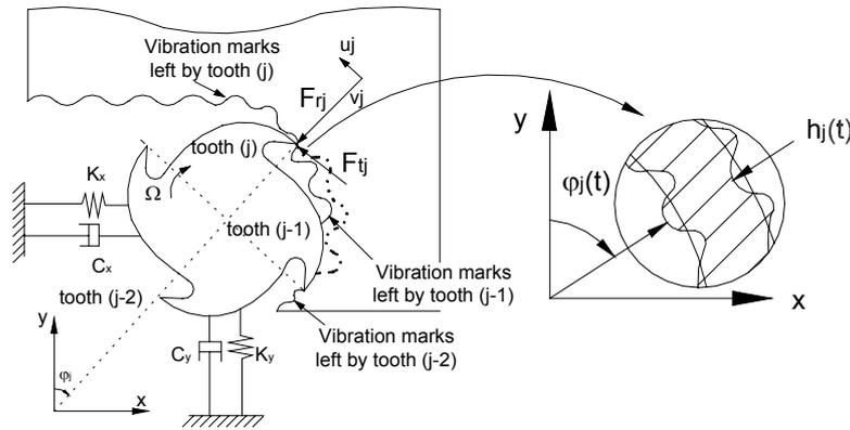
Figure 1 – Schematic of milling operation
