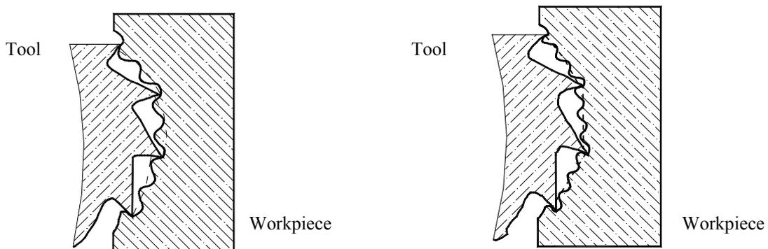
Figure 9 – Waves between teeth, left (2 waves) and right (3 waves)
