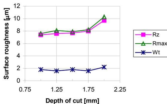
Figure 6. Surface roughness in function of the depth of cut for a spindle rotation  $n = 13.922$  rpm
