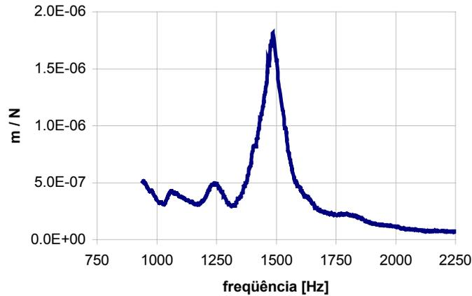
Figure 2. Transfer function of the endmill, L/D= 4.7.
