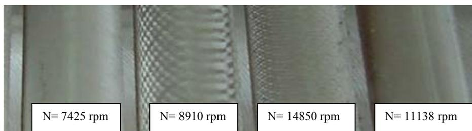
Figure 4. Machined surfaces for stable and unstable cuts
