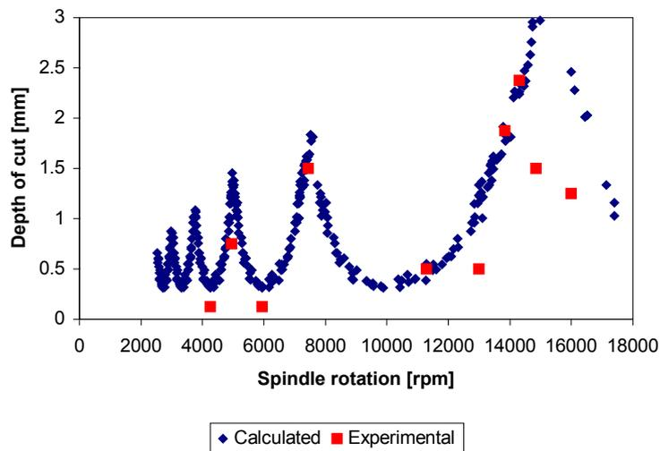
Figure 10. Simulated stability lobe diagram
