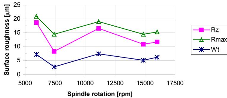
Figure 5. Surface roughness in function of the spindle rotation for a 6 flute endmill.
