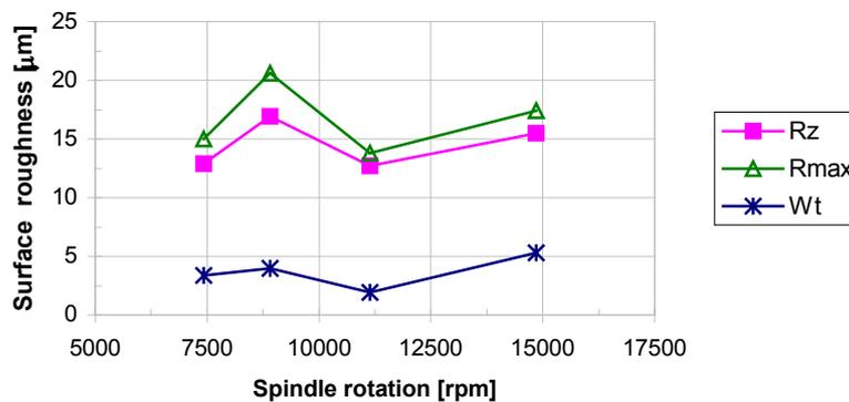
Figure 3. Surface roughness in function of the spindle rotation for a 4 flute endmill.
