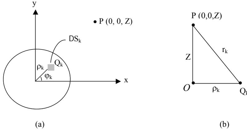
Figure 4. Circular disk – (a) disk is on the plane  $(x, y)$ , (b) the distance between the element of the surface, containing a point  $Q_k$ , and the point  $P$ .
