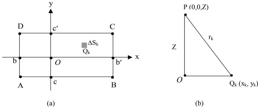
Figure 2. Rectangular plate – (a) rectangular plate is on the plane  $(x, y)$ , (b) the distance between the element of the surface, containing a point  $Q_k$ , and the point  $P$ .
