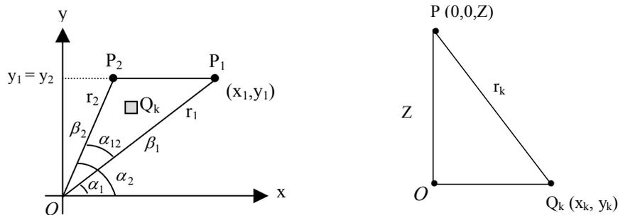
Figure 3. Triangular plate – (a) Triangle  $\overline{OP_1P_2}$  located in the xy-plane (x, y), (b) the distance between the element of the surface, containing a point Q<sub>k</sub>, and the point P.
