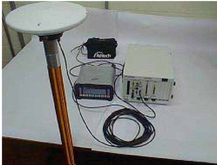
Figure 2. GPS antenna, Z-12 receiver, battery and computer
