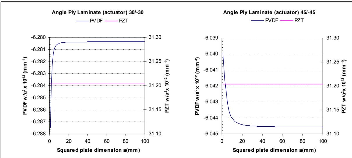
Figure 3. Transverse deflection of angle-ply laminates for prescribed unit potential difference (PZT and PVDF).
