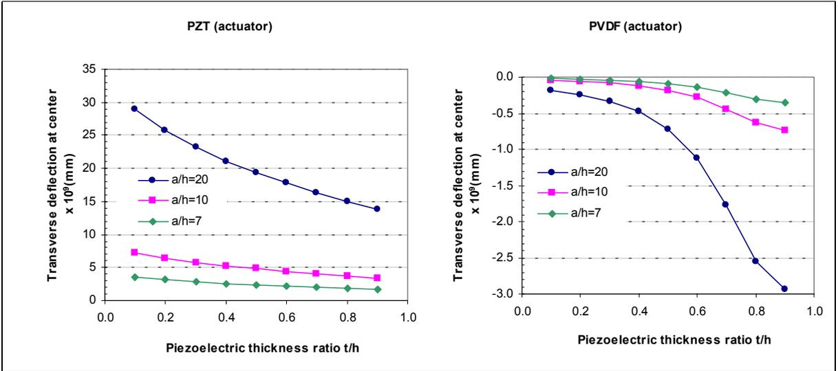
Figure 2. Transverse deflection *versus* piezoelectric thickness ratio for prescribed unit potential difference (PZT and PVDF).
