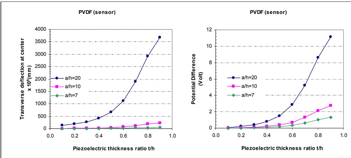
Figure 5. Transverse deflection and potential *versus* piezoelectric thickness ratio for a distributed unit load (PVDF).
