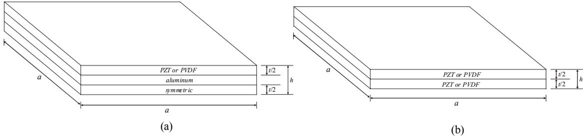
Figure 1.(a): three-layer symmetric cross-ply laminate. (b): two-layer antisymmetric angle-ply laminate.
