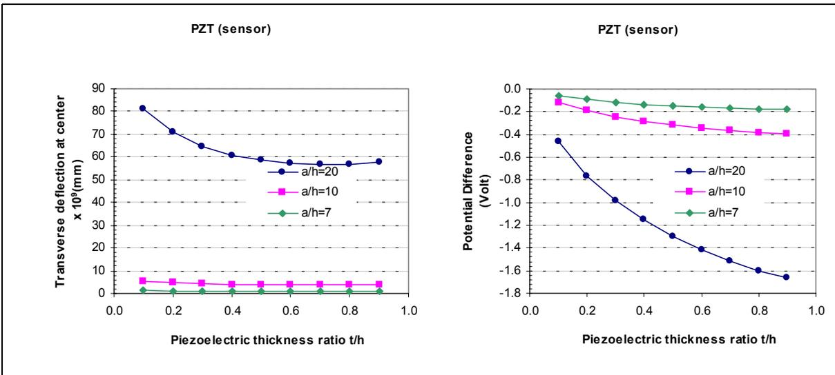
Figure 4. Transverse deflection and potential *versus* piezoelectric thickness ratio for a distributed unit load (PZT).
