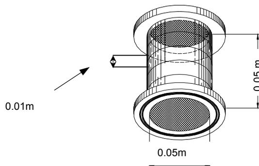
Figure 3. Scheme of the drying cell used for obtaining moisture distribution throughout the bed.
