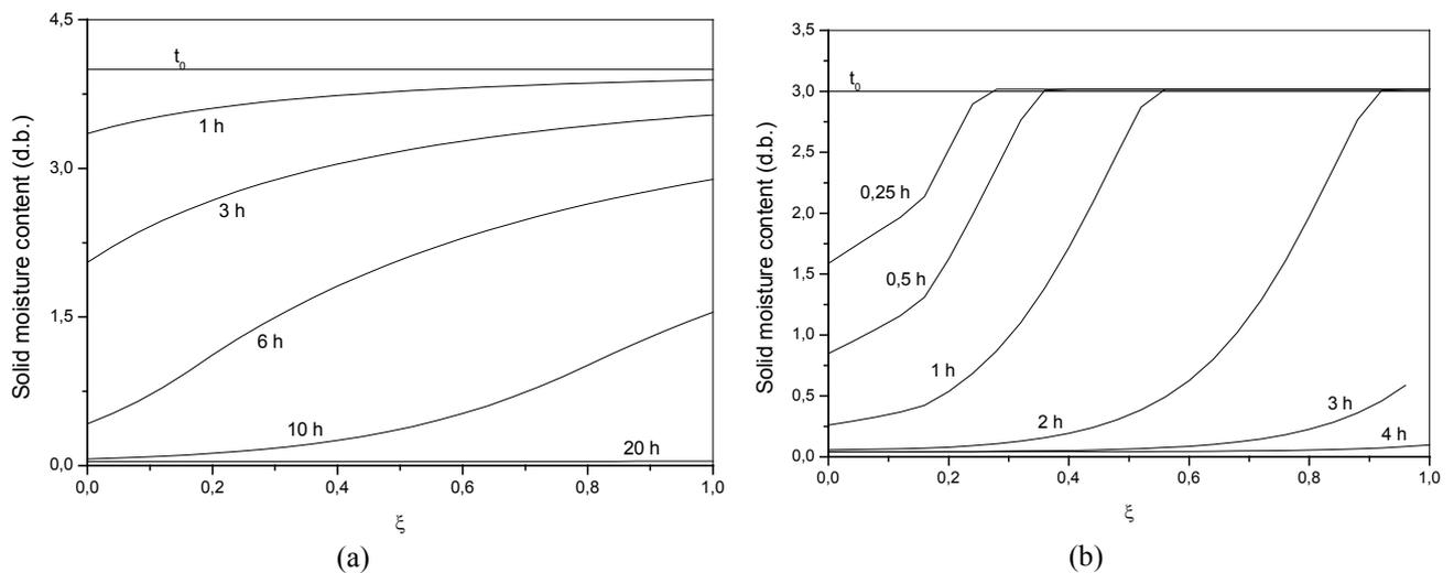
Figure 8. Simulated moisture content profiles throughout the packed bed during drying at  $T_{g0}=50^{\circ}\text{C}$  and  $v_g=0,5$  m/s. (a) for particles with mucilage and (b) for particles without mucilage.
