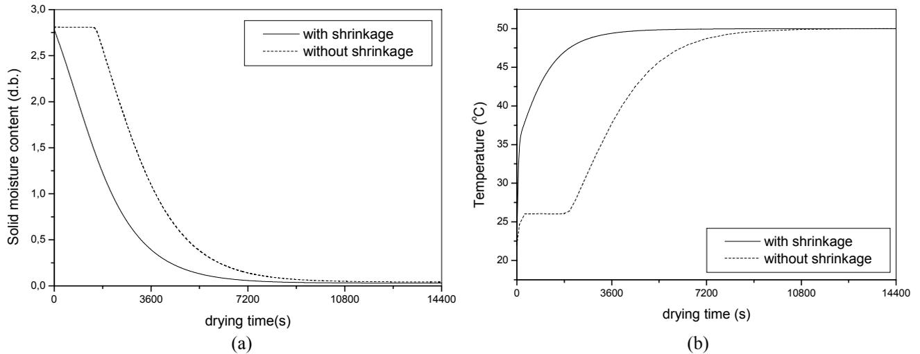
Figure 7. Predicted results as function of drying time at  $z=0.01$  m;  $T=50^{\circ}\text{C}$ ;  $v_g=0.5$  m/s, for particles without mucilage, with and without consideration of shrinkage effect. (a) Moisture content, (b) Temperature of the solid.
