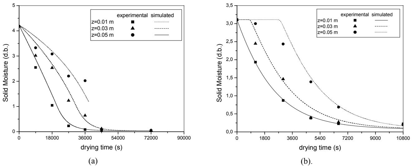
Figure 5. Experimental and predicted moisture content as a function of time at three bed heights during drying at  $T_{g0}=50^{\circ}\text{C}$  and  $v_g=0.5\text{ m/s}$ . (a) for particles with natural coat, (b) for particles without natural coat.
