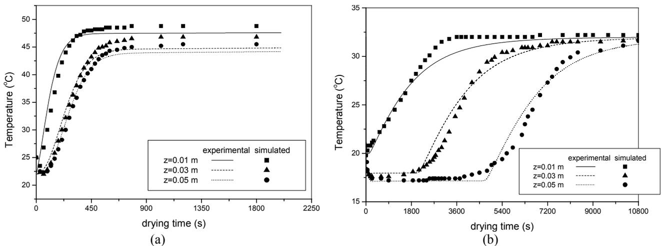
Figure 6. Experimental and predicted temperature values versus time at three bed heights during drying at  $v_g=0.5\text{ m/s}$ . (a) for particles with natural coat and  $T_{g0}=50^{\circ}\text{C}$ ; (b) for particles without natural coat and  $T_{g0}=32^{\circ}\text{C}$ .
