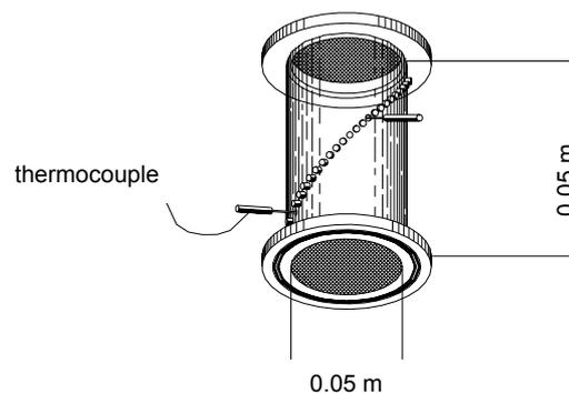
Figure 4. Scheme of the drying cell constructed for obtaining of temperature distribution and shrinkage measurements.
