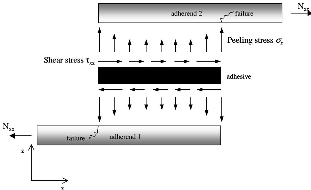
Figure 5. Peeling and shear stresses in single lap joint.
