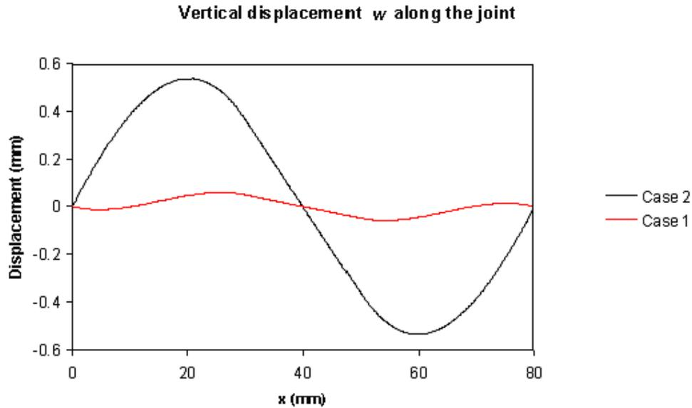
Figure 11. Vertical displacement  $w$  along the joint for cases 1 and 2 in coupling effect study.
