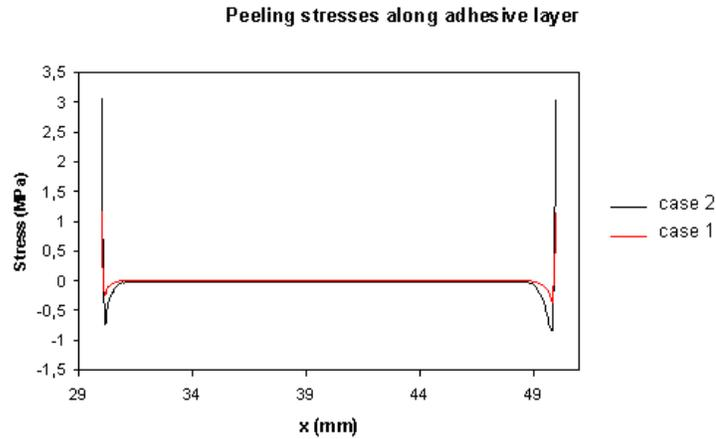
Figure 9. Peeling stresses along adhesive layer for cases 1 and 2 in coupling effect study.
