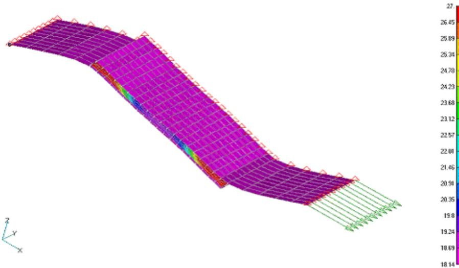
Figure 15. Deformed shape and peeling stress along the adhesive layer in non-linear analysis.
