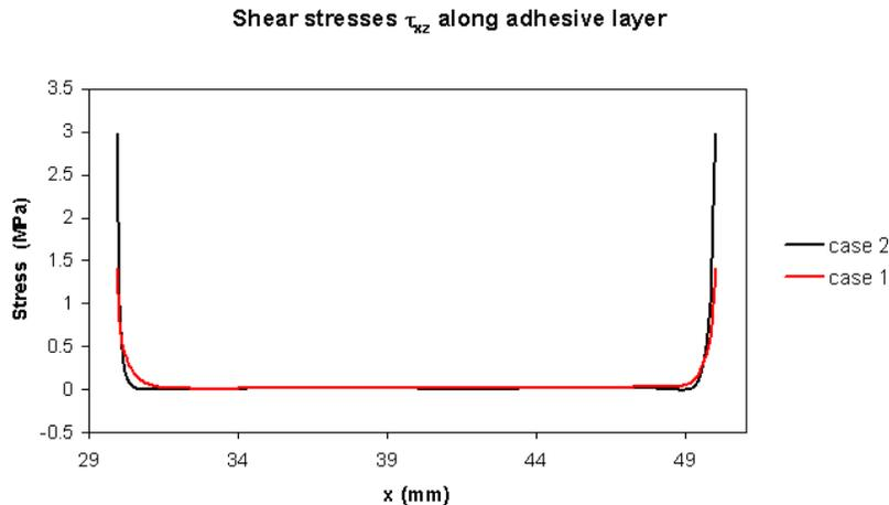
Figure 10. Shear stresses  $\tau_{xz}$  along adhesive layer for cases 1 and 2 in coupling effect study.
