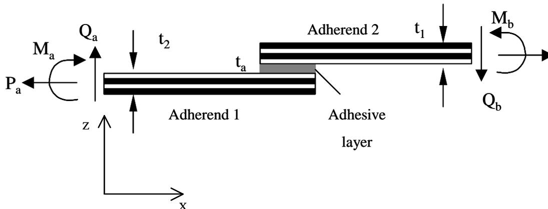
Figure 1. Schematic illustration of adhesive single lap joint subjected to general loading conditions.
