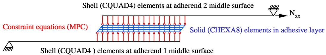
Figure 4. Single lap joint FEM.
