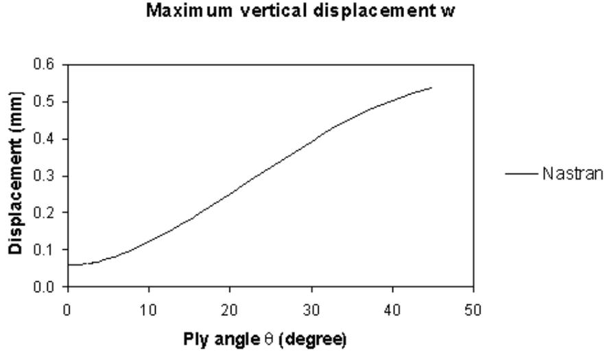
Figure 7. Maximum vertical displacements of adherends as function of ply angle  $\theta$ .
