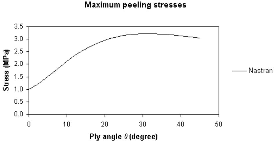
Figure 8. Maximum peeling stresses of adhesive as function of ply angle  $\theta$ .
