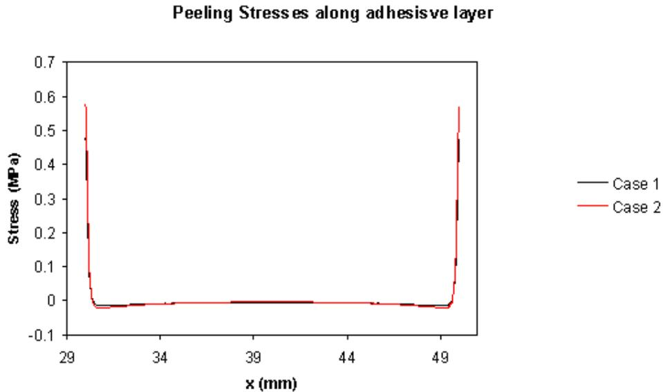
Figure 12. Peeling stresses along adhesive layer for cases 1 and 2 in stacking sequence study.
