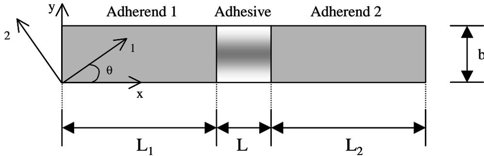
Figure 6. Single lap joint : basic dimensions and laminate coordinate system.
