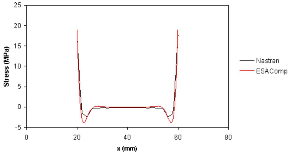
Figure 14. Peeling stress along adhesive layer in non-linear analysis.
