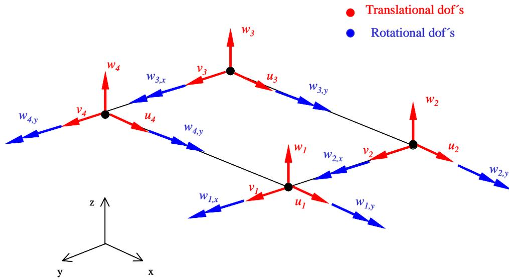
Figure 2. CQUAD4 plate element with corresponding degrees of freedom.
