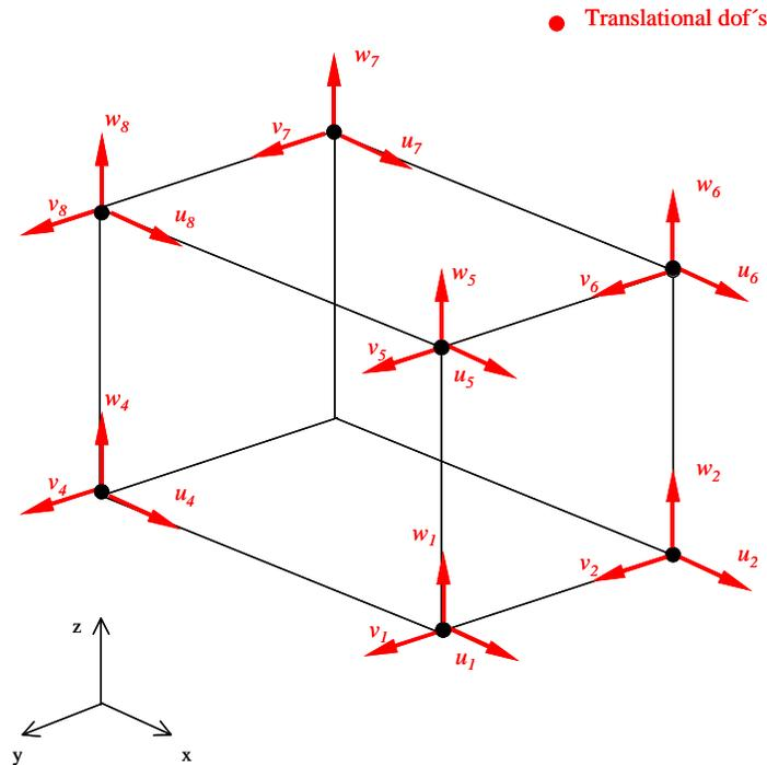
Figure 3. CHEXA8 solid element with corresponding degrees of freedom.
