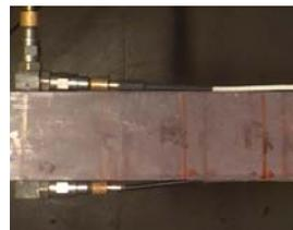
Figure 3. Measurement all consisting of 3 accelerometers.
