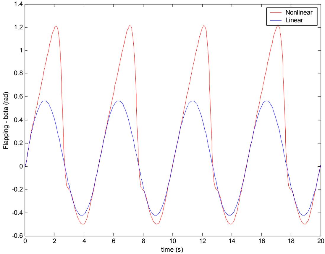
Figure 1. Nonlinear and linear gust / collective pitch response.
