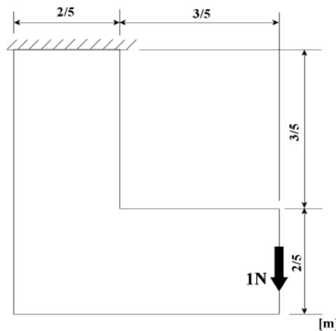
Figure 5. Geometry of L beam problem
