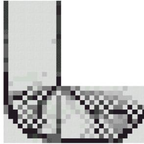
Figure 4. Example of checkerboard pattern
