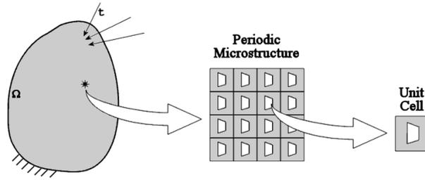
Figure 1. Representation of a composite material made of a periodic microstructure
