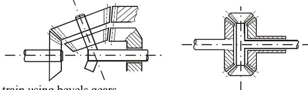
Figure 3 Planetary gear train using bevels gears
