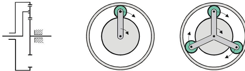
Figure 5. Example of the simple PGT
