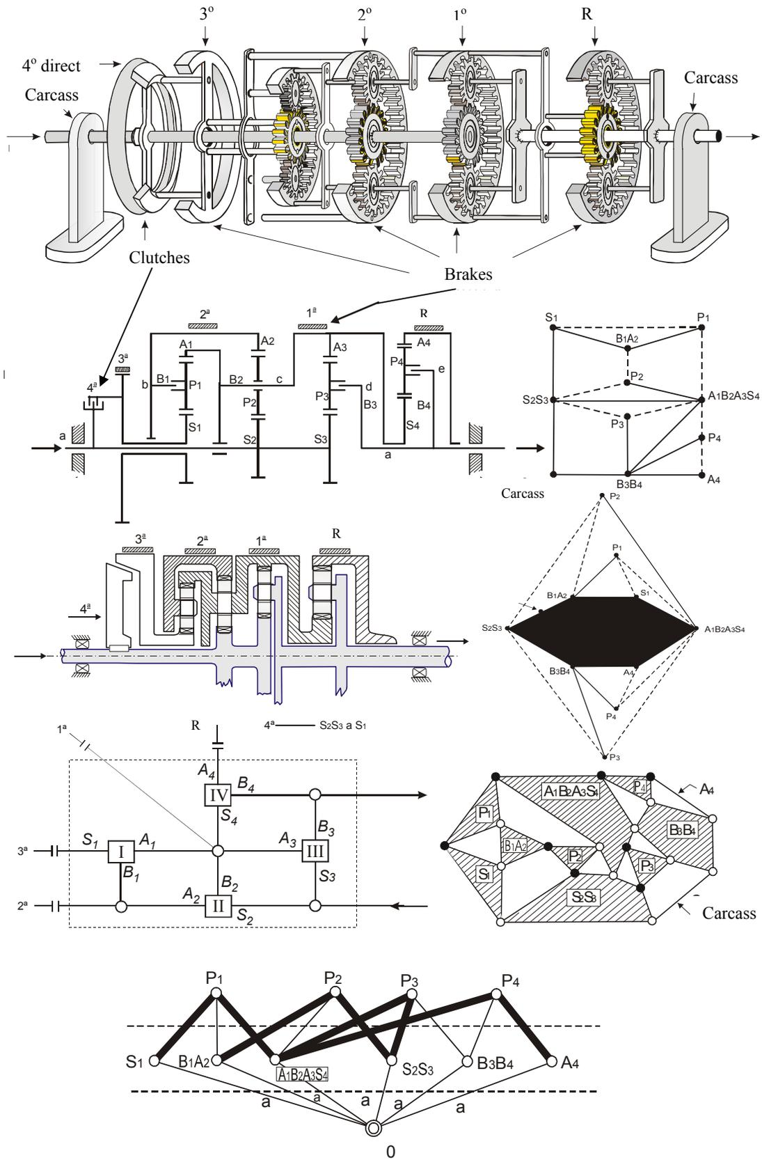
Figure 16. Example of application of the PGTs representation forms using “Wilson Transmission”
