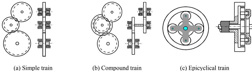
Figure 1. Types of the gear trains.
