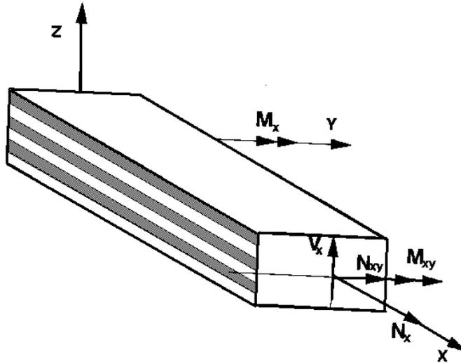
Figure 1. Laminated beam, with force and moment resultants
