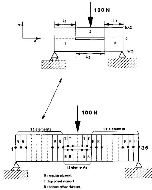
Figure 8. Simply supported beam
