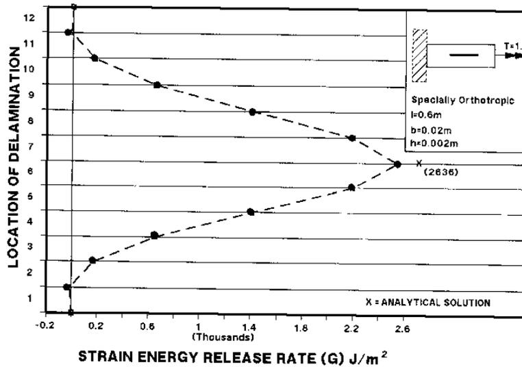
Figure 7. Strain energy release rate for cantilever beam
