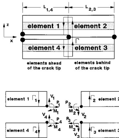
Figure 2. zero-volume path for J-integral
