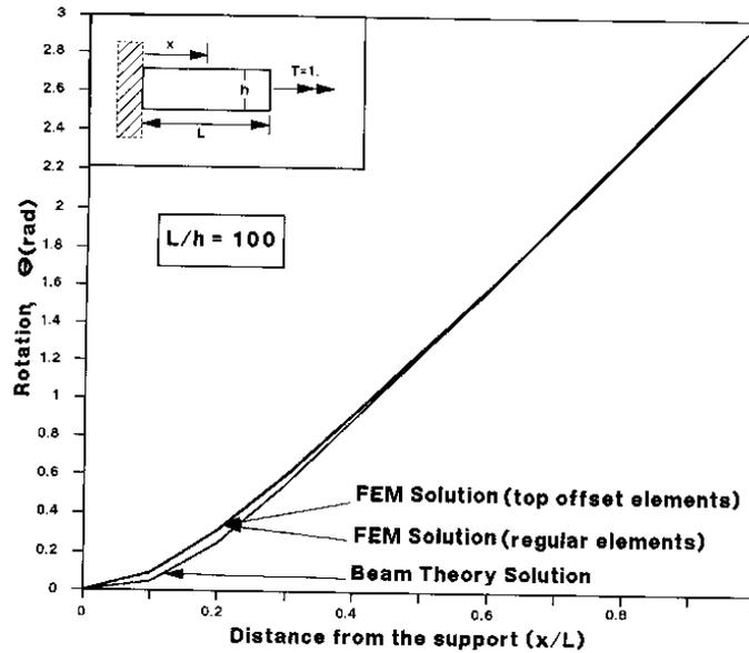
Figure 4. Angle of twist along the length ( $L / h = 100$ )
