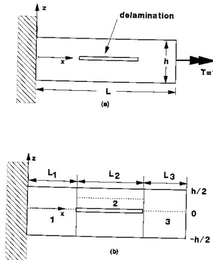
Figure 5. Delaminated beam: (a) Under torsion (b) Separated by parts
