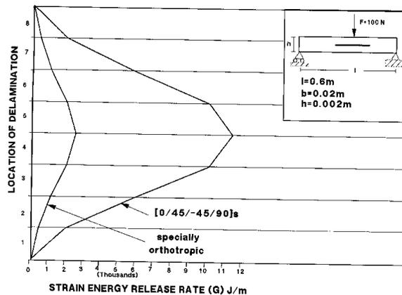
Figure 9. Strain energy release rate for simply supported beam
