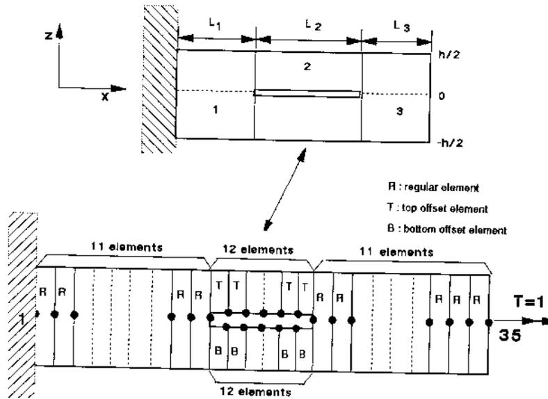
Figure 6. Delamination close to the top plane
