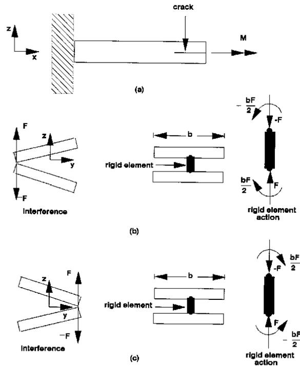
Figure 3. Rigid elements: (a) beam under torsion (b) interference on left side (c) (b) interference on right side
