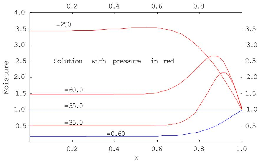
Figure 3. Evolution of moisture profiles during the process
