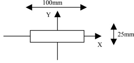
Figure 1 Geometry and coordinate system for contact drying for a moisture porous sheet.
