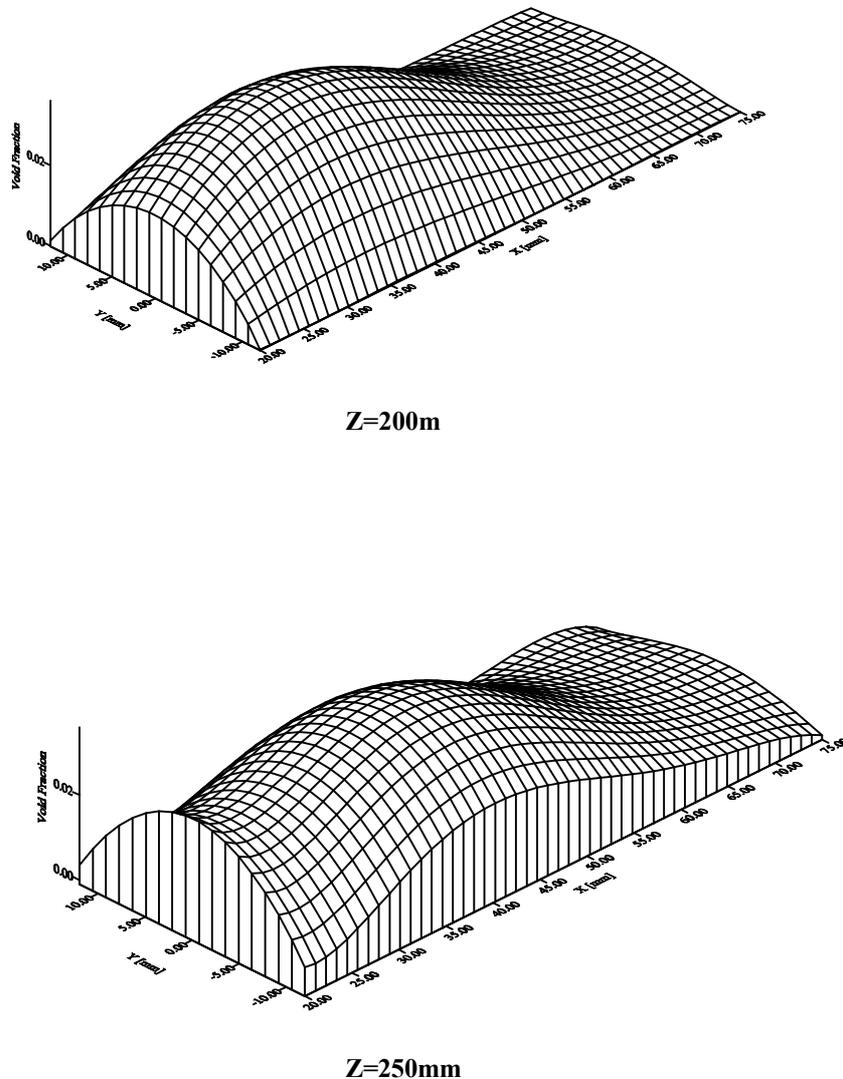
Figure 5. Tri-dimensional void-fraction profiles.
