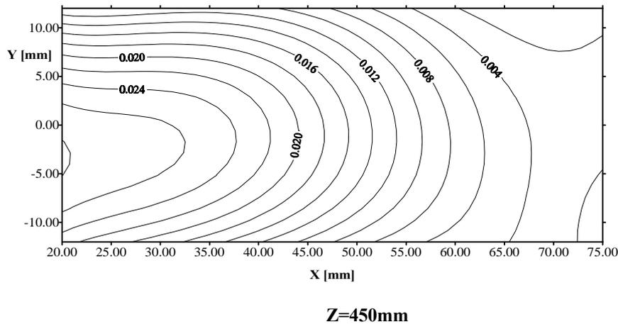
Figure 6. (Continued). Contour lines of void fraction profiles. Plate shows plane defined by  $Z=450$  mm.
