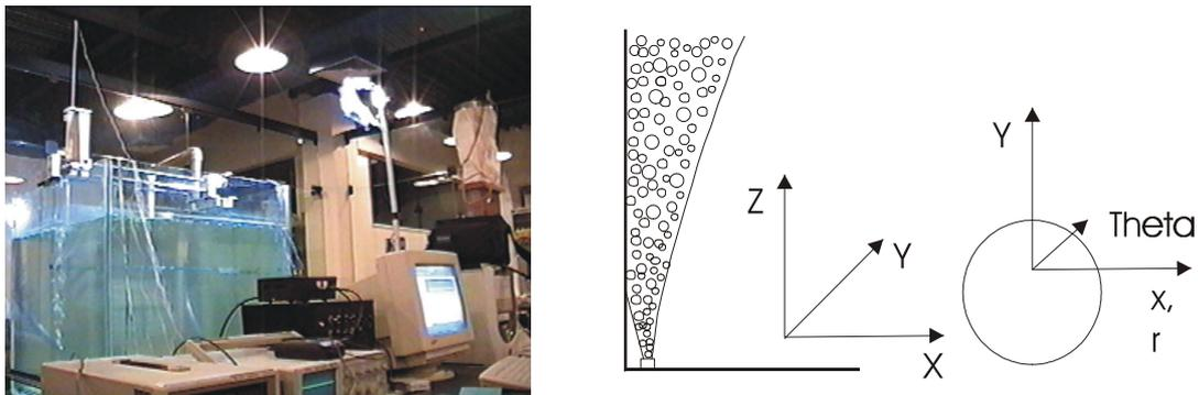
Figure 1. Picture of water tank and sketch of bubble plume near a wall with the coordinate system.
