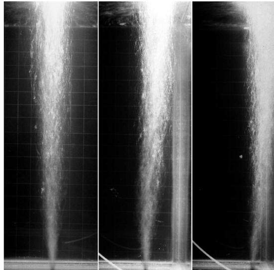
Figure 3. General flow pattern showing plume behaviour near to a wall.
