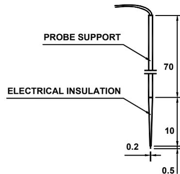
Figure 2. Picture of calibration set up and of the electro-conductivity sensor. Dimensions are in mm.
