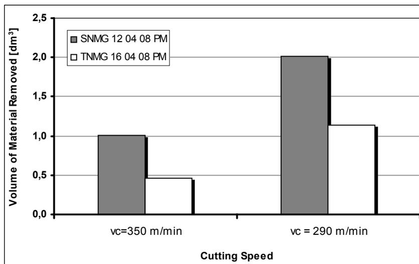
Fig. 1 – Tool life in volume of material removed vs tool geometry for tests with  $f = 0,4$  mm/rot,  $a_p = 2$  mm and P25 carbide class
