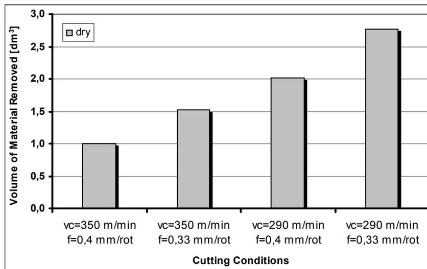
Fig. 2 – Tool life in volume of material removed vs cutting conditions for tests with  $a_p = 2$  mm and P25 carbide class
