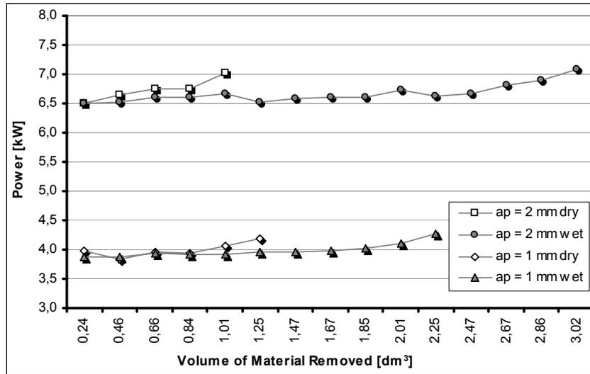
Fig. 7 –Consumed Power (kW) vs volume of material removed for tests with  $v_c = 350 \text{ m/min}$ ,  $f = 0,4 \text{ mm/rot}$  and P25 carbide class
