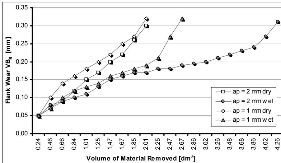
Fig. 6 –Flank wear  $VB_B$  vs volume of material removed for tests with  $v_c = 350$  m/min,  $f = 0,4$  mm/rot and P15 carbide class
