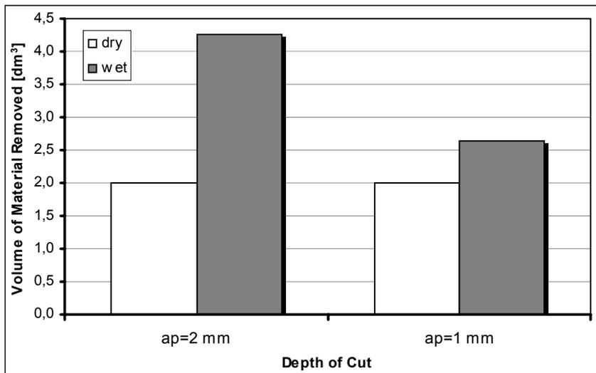
Fig. 4 – Tool life in volume of material removed vs depth of cut ( $a_p$ ) for tests with  $v_c = 350$  m/min,  $f = 0,4$  mm/rot and P15 carbide class
