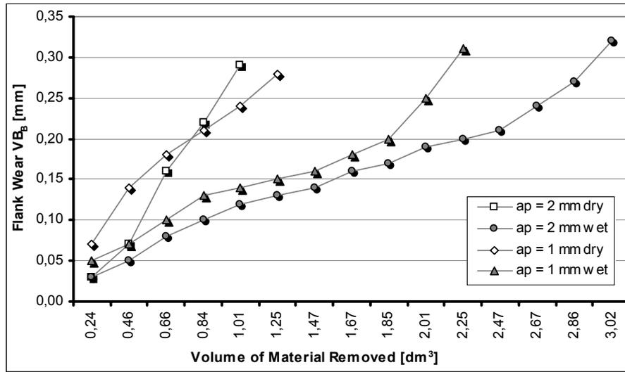
Fig. 5 –Flank wear  $VB_B$  vs volume of material removed for tests with  $v_c = 350$  m/min,  $f = 0,4$  mm/rot and P25 carbide class
