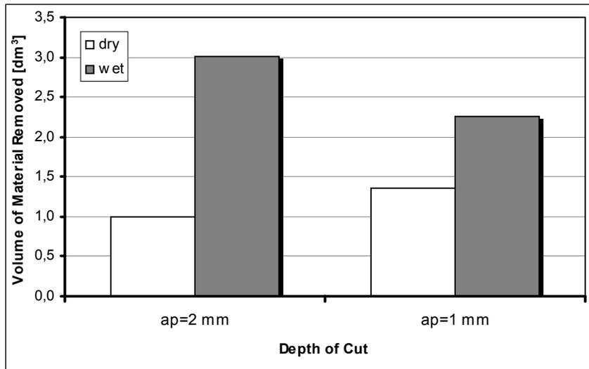
Fig. 3 – Tool life in volume of material removed vs depth of cut ( $a_p$ ) for tests with  $v_c = 350$  m/min,  $f = 0,4$  mm/rot and P25 carbide class
