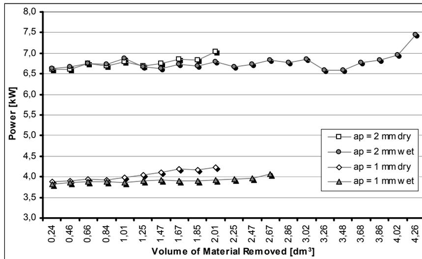
Fig. 8 –Consumed Power (kW) vs volume of material removed for tests with  $v_c = 350 \text{ m/min}$ ,  $f = 0,4 \text{ mm/rot}$  and P15 carbide class
