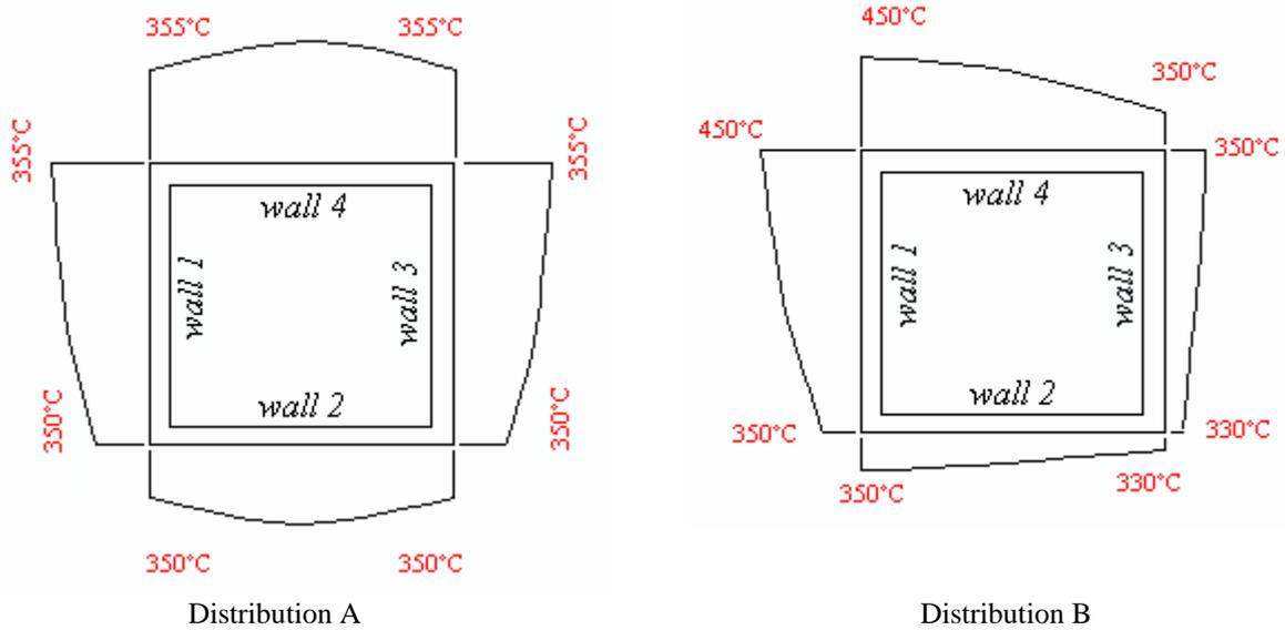
Figure 4. Wall temperature distributions.
