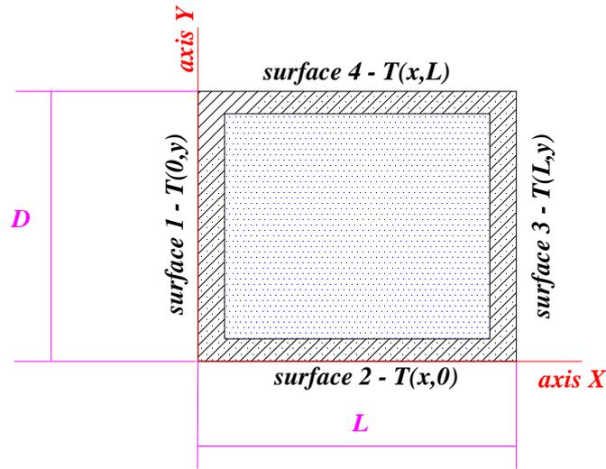
Figure 2. Duct cross-section and variable wall temperature distribution schematics.
