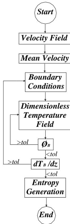
Figure 3 - Computational Model Flowchart.
