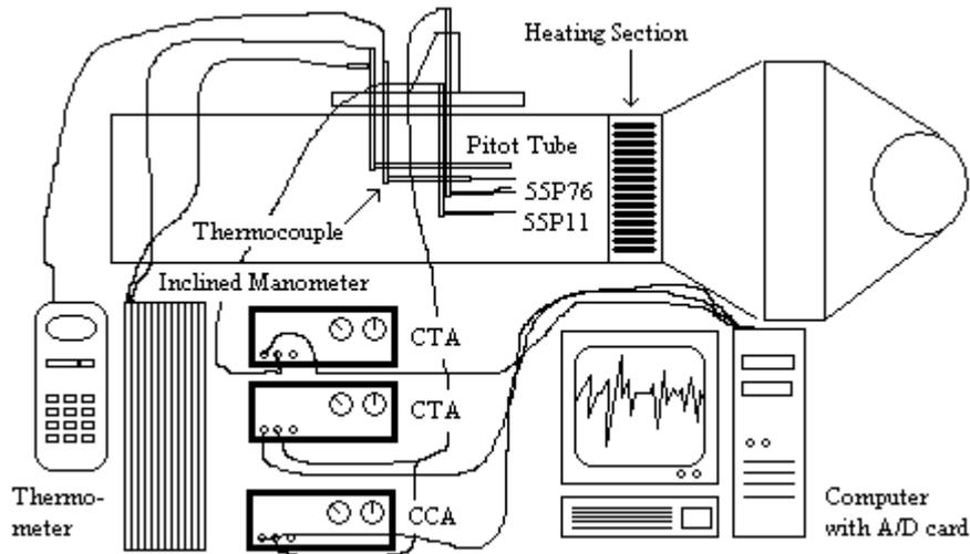
Figure 2. Position of probes in the wind tunnel.
