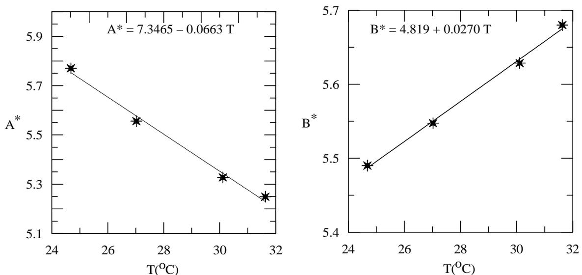
Figure 3. The variation of the calibration parameters  $A^*$  and  $B^*$  with the fluid temperature.
