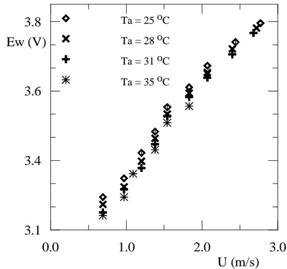
Figure 4. Dependence of velocity measurements on the ambient fluid temperature.
