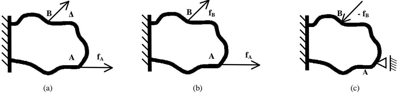
Figure 1. (a) Problem statement; (b) Kinematic requirement; (c) Structural requirement.
