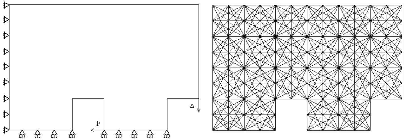
Figure 4. Initial design domain for a compliant gripper.
