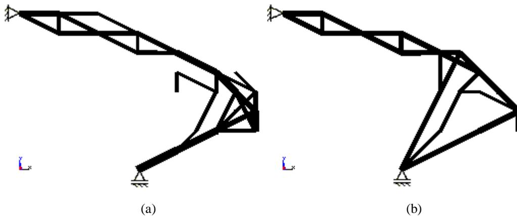
Figure 5. Compliant gripper design: (a)  $p=1.0$ ; (b)  $p=1.8$ .
