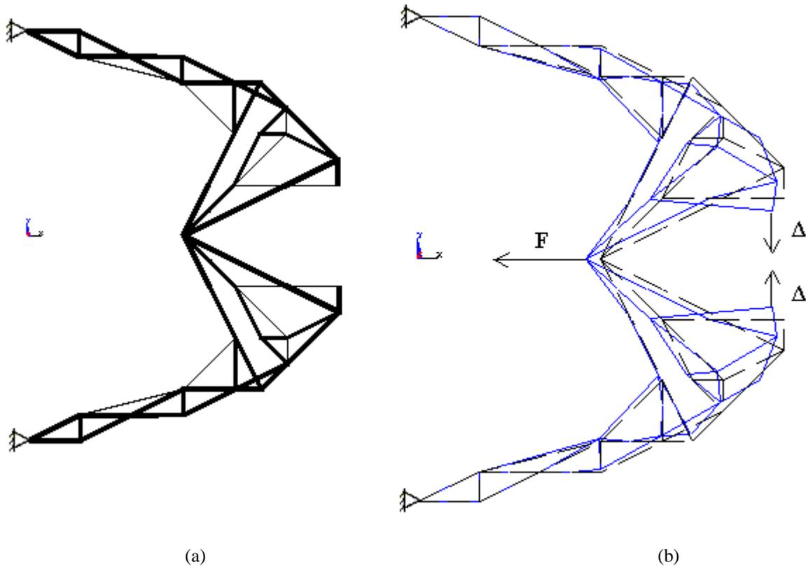
Figure 6: (a) Interpretation of the obtained topology. (b) Finite element simulation of the entire gripper. In continuous lines, the deformed shape.
