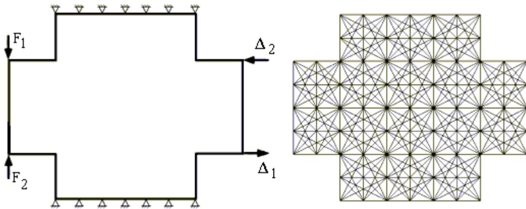
Figure 8. Initial design domain for multi-flexible mechanism.
