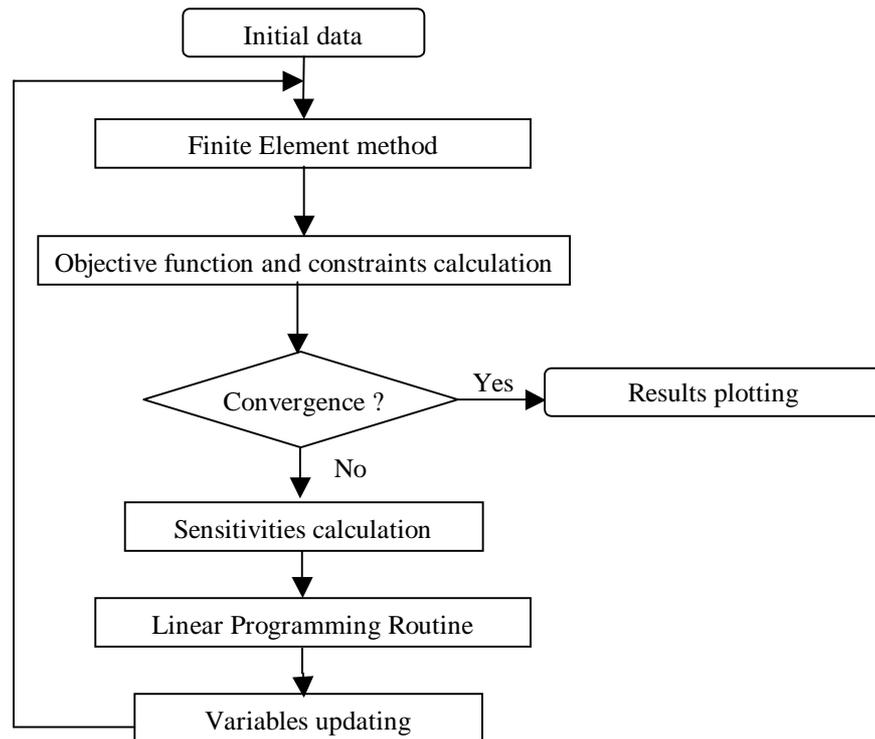
Figure 3. Flowchart of the iterative optimization process.
