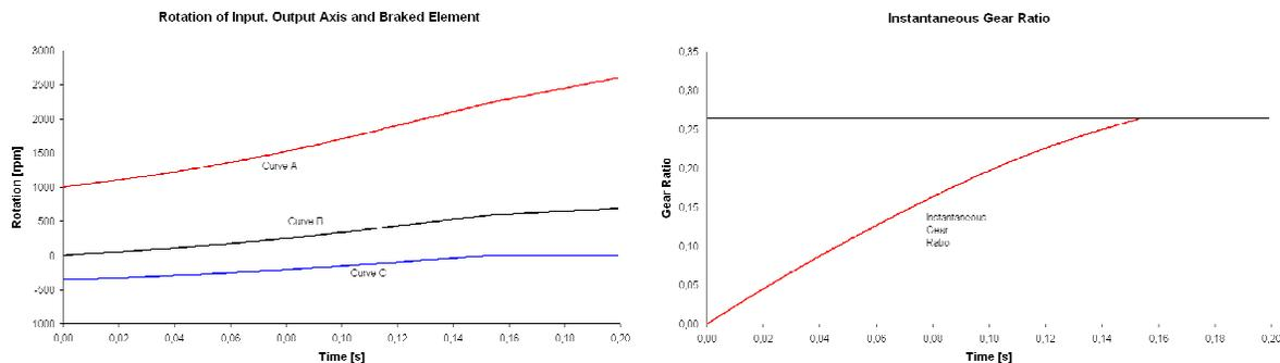
Figure 4. Variation of the speed of the main components for the first gear in the simulation.
