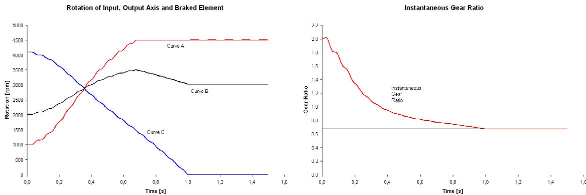
Figure 9. Variation of the speed of the main components for the third gear of the Wilson gearbox when the loading is applied.
