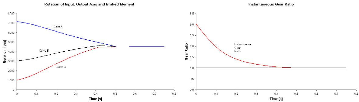
Figure 10. Variation of the speed of the main components for the fourth gear in the simulation.
