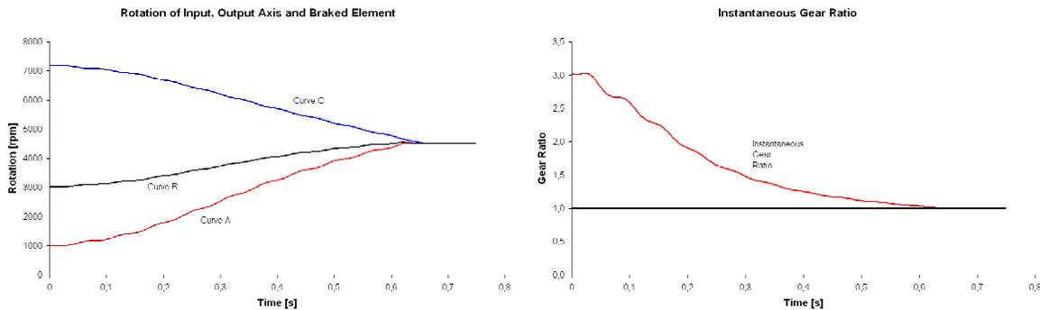
Figure 11. Variation of the speed of the main components for the fourth gear of the Wilson gearbox when the loading is applied.
