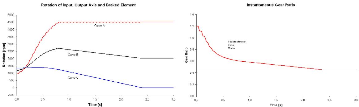
Figure 7. Variation of the speed of the main components for the second gear of the Wilson gearbox when the loading is applied.
