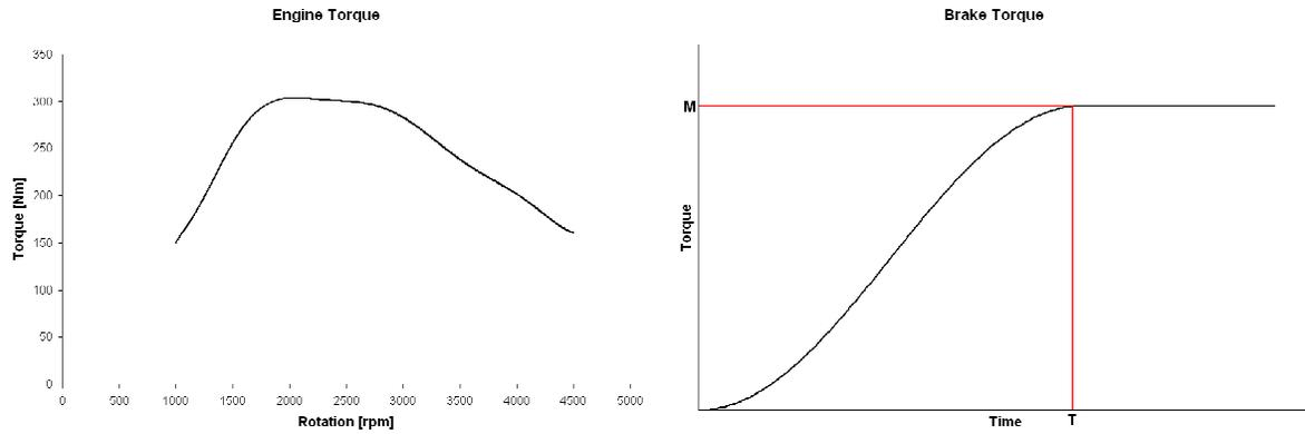
Figure 3. The engine torque curve and the schematic brake torque curve used in the simulation.
