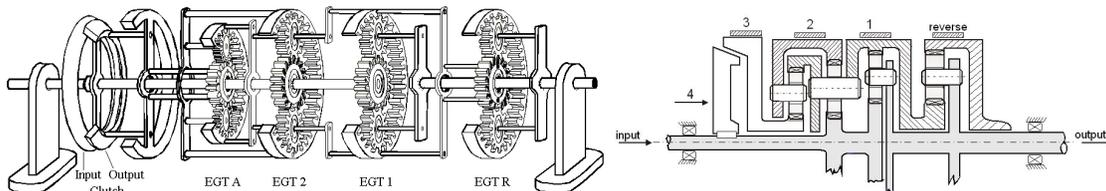
Figure 1. The components of the Wilson Gearbox and the components used to set the gears and sketch of the Wilson Gearbox
