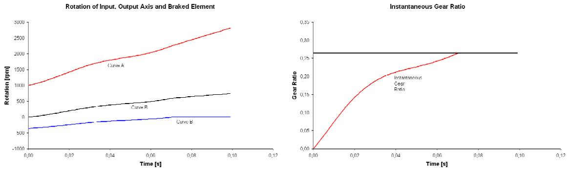
Figure 5. Variation of the speed of the main components for the first gear of the Wilson gearbox when the loading is applied.
