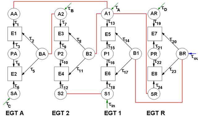
Figure 2. Torque flow diagram of the Wilson Gearbox
