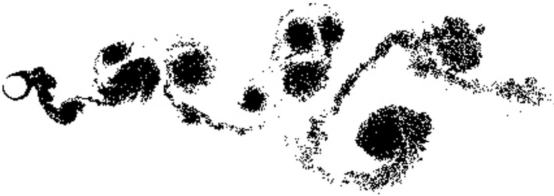
Figure 7. Positions of the wake vortices for  $Re = 10^5$ , at  $t = 50.0$ ;  $N = 64$ ,  $\Delta t = 0.05$  and  $\varepsilon = \sigma_0 = 0.0045$  using PMA.
