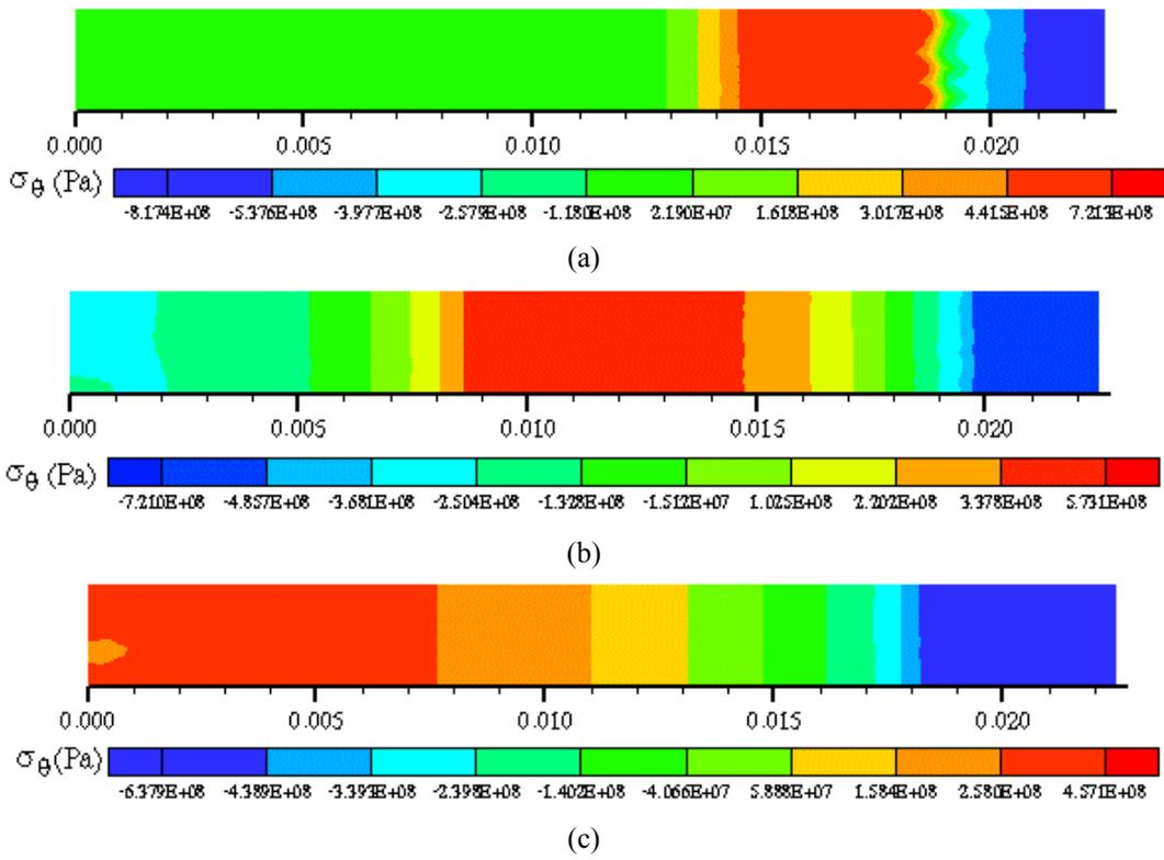
Figure 5. Residual stress  $\sigma_{\theta}$  distribution for different  $e_{PI}$ : (a) 3.5 mm; (b) 8.0 mm; (c) 11.0 mm.
