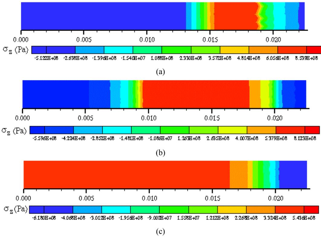
Figure 6. Residual stress  $\sigma_z$  distribution for different  $e_{pi}$ : (a) 3.5 mm; (b) 8.0 mm; (c) 11.0 mm.
