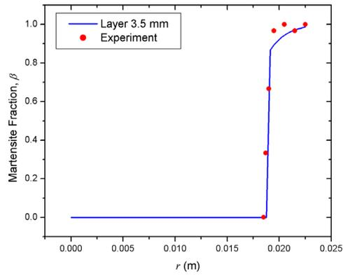
Figure 4. Comparison between numerical and experimental results: Volumetric fraction of martensite for  $e_{PI} = 3.5$  mm (Pacheco et al., 2001a; Pacheco et al., 2001b; Camarão, 1998).
