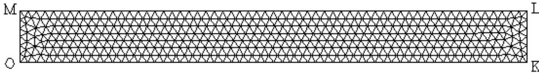
Figure 2. Mesh employed for finite element analysis.
