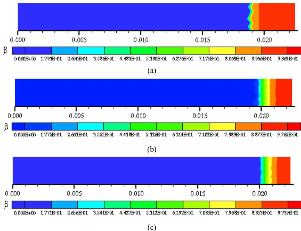
Figure 3. Volumetric fractions of martensite: (a)  $e_{pl} = 3.5$  mm; (b)  $e_{pl} = 8.0$  mm; (c)  $e_{pl} = 11.0$  mm.
