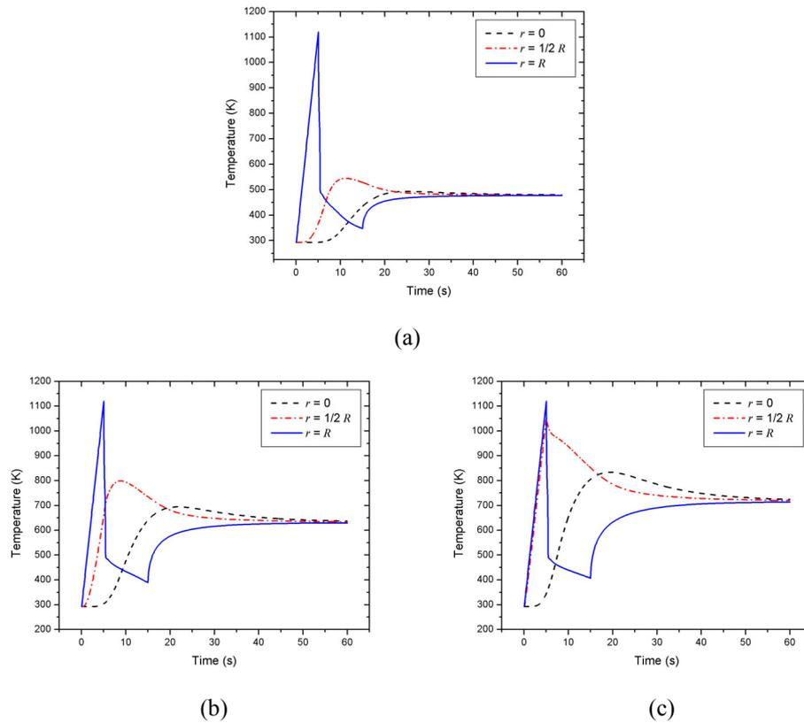
Figure 8. Time history of temperature for different radius positions and  $e_{pl}$ : (a) 3,5 mm; (b) 8,0 mm; (c) 11,0 mm.
