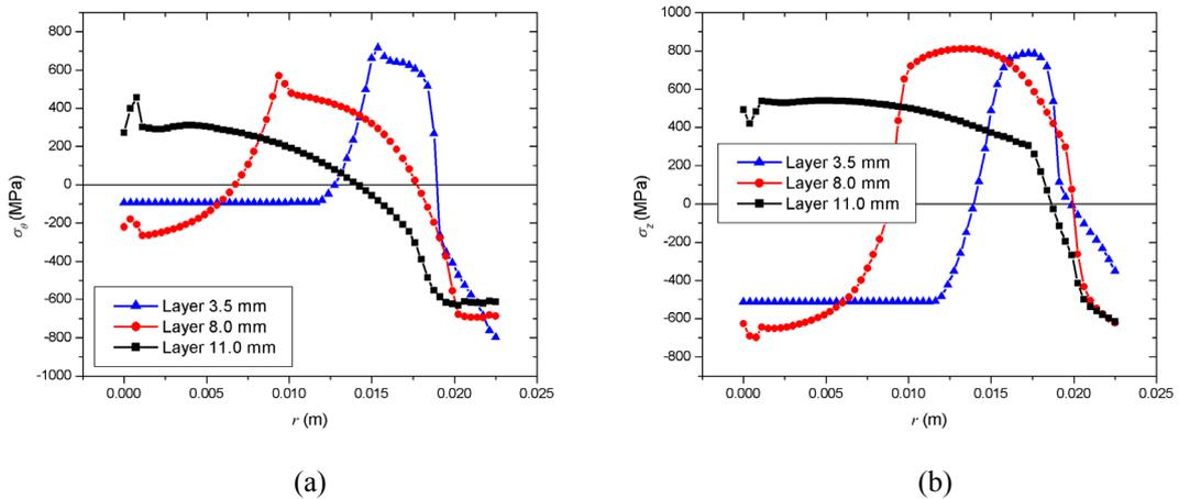
Figure 7. Residual stress distribution over the radius for the final time instant. (a)  $\sigma_\theta$ ; (b)  $\sigma_z$ .
