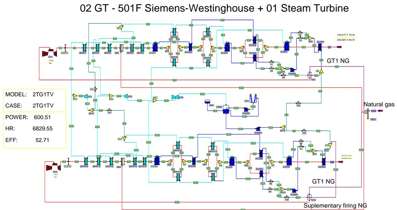
Figure 3. Thermal scheme of a combined cycle plant and the results of the design point simulation
