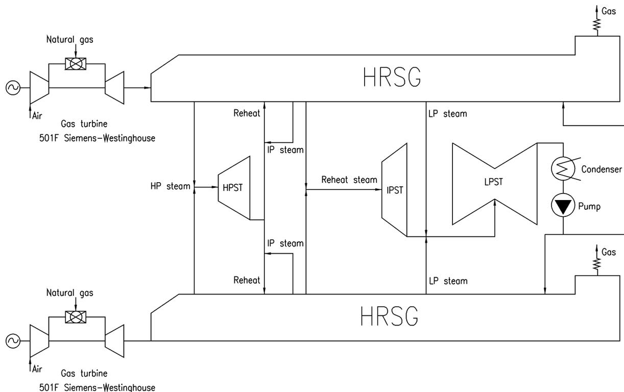
Figure 1 – Combined cycle plant simplified thermal scheme
