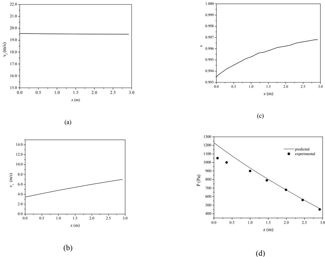
Figure 1. Graphs of (a) fluid velocity, (b) particle velocity, (c) voidage and (d) pressure as functions of axial position, glass spheres,  $d_p=1.10$  mm,  $W_s=0.124$  kg/s;  $W_f=0.0414$  kg/s;  $L=2.88$  m and  $D_t=53.4$  mm.
