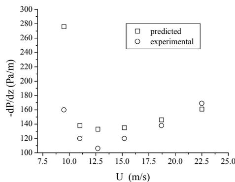
Figure 3. Experimental and predicted pressure gradients versus air velocity in the transport tube, glass spheres,  $d_p=1.00$  mm;  $W_s=0.041$  kg/s (experimental data from Narimatsu, 2000).
