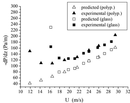
Figure 5. Predicted and experimental pressure gradients as functions of air velocity for glass spheres ( $\rho_p=2500$  kg/m<sup>3</sup>) and polipropylene beads ( $\rho_p=935$  kg/m<sup>3</sup>);  $d_p=3.68$  mm;  $W_s=0.037$  kg/s.
