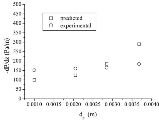
Figure 4. Experimental and predicted pressure gradients as functions of the particle diameter;  $U=22$  m/s and  $W_s=0.042$  kg/s.
