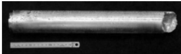
Figure 4. AA6070 aluminum alloy billet obtained by horizontal continuous casting.
