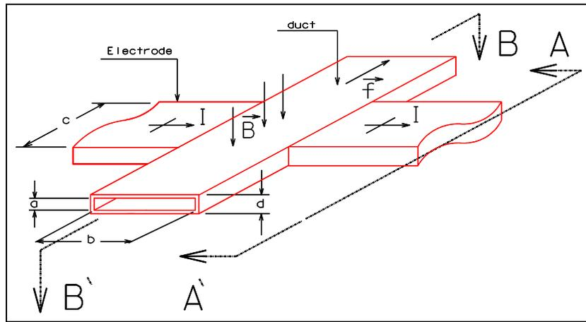
Figure 1. The principle of operation of a DC electromagnetic pump.
