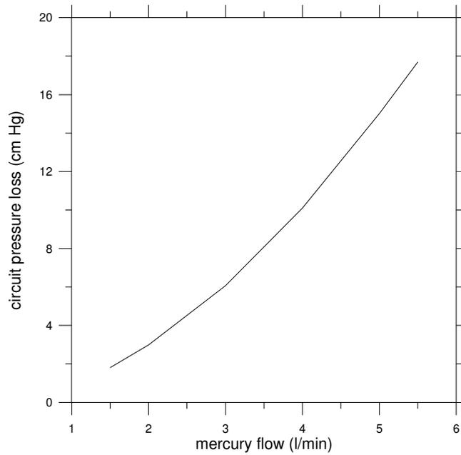
Figure 7. BEMC-1 theoretical loop pressure loss data.
