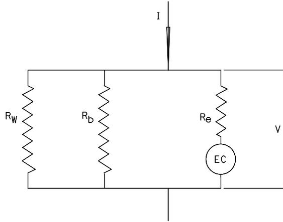
Figure 2. Equivalent electric circuit of the DC electromagnetic pump.
