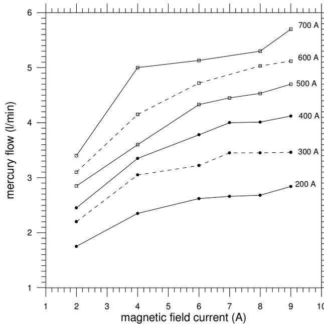
Figure 8. Experimental fluid flow data of the DC electromagnetic pump.
