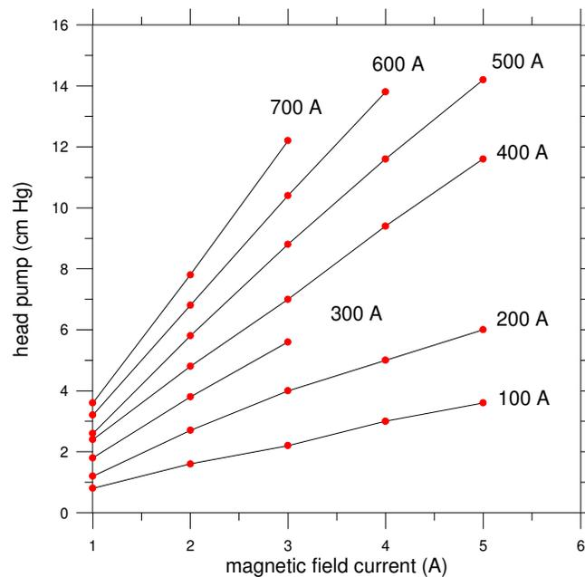
Figure 6. Experimental static pressure data of the DC electromagnetic pump.
