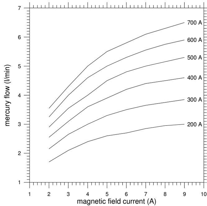
Figure 9. BEMC-1 theoretical fluid flow data of the DC electromagnetic pump.
