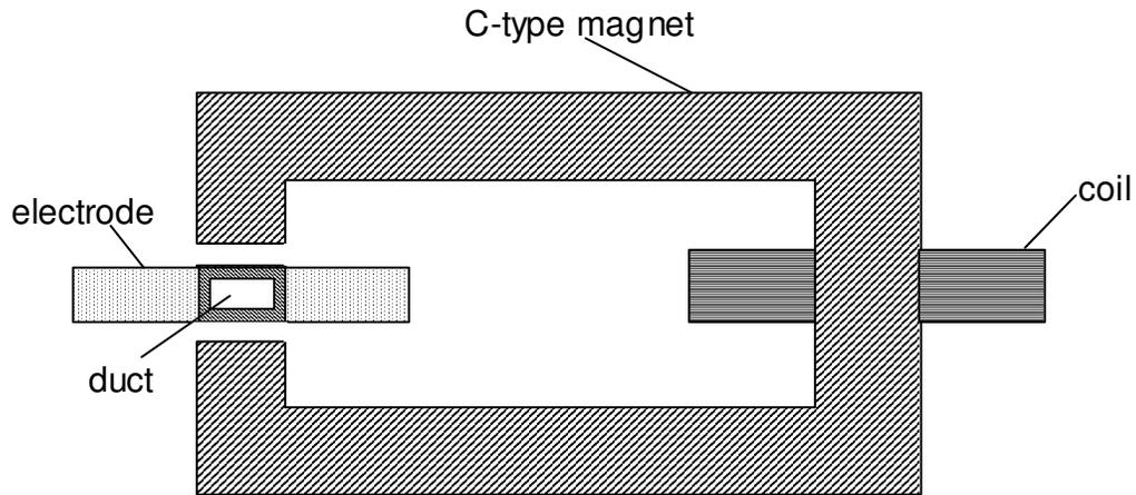
Figure 3. Cross section of the DC electromagnetic pump with C-type magnet.
