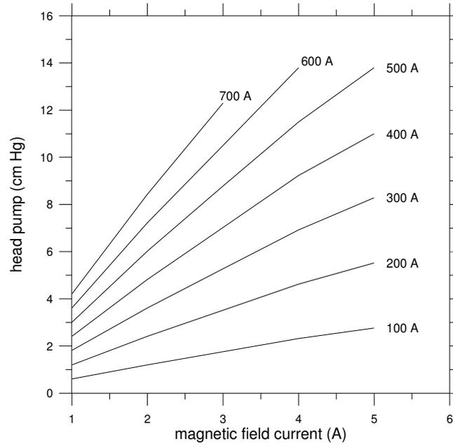
Figure 5. BEMC-1 theoretical static pressure data of the DC electromagnetic pump.
