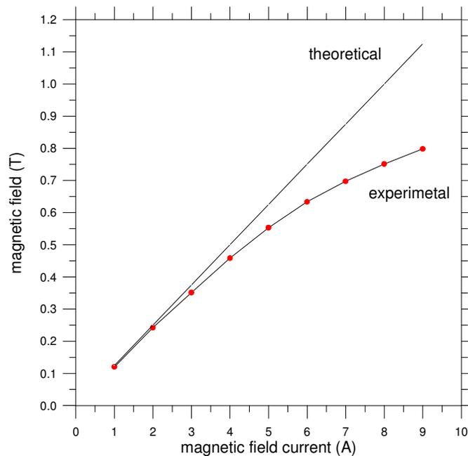
Figure 4. Magnetic field in the center of the air gap of the C-type magnet.
