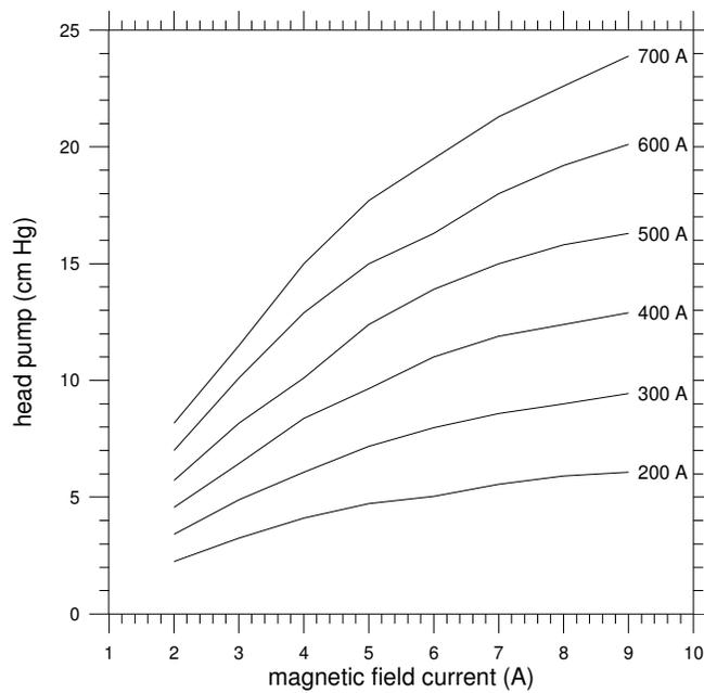
Figure 10. BEMC-1 theoretical dynamic head pump.
