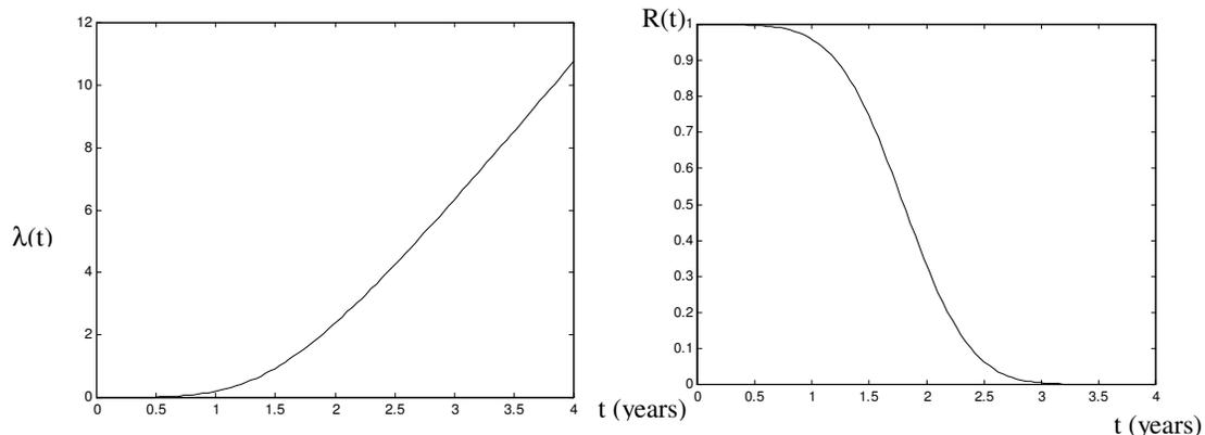
Figure 5. Reliability and Failure Rate for the Hydraulic Actuator.
