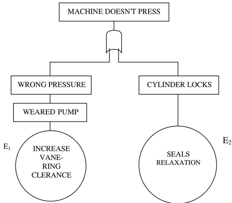
Figure 6. Fault Tree to the Deep Drawing Press Hydraulic System.
