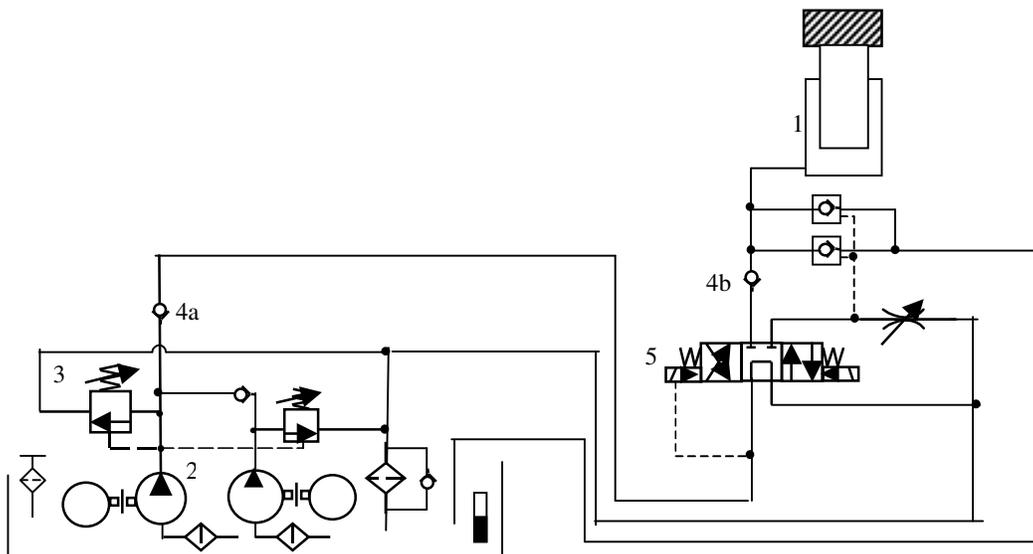
Figure 2. Dual Hydraulic Circuit for a 250 ton Press.
