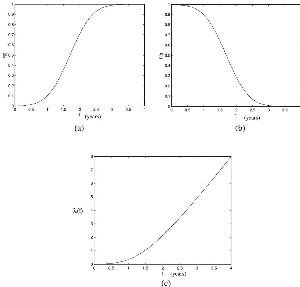
Figure 3. (a) Cumulative Distribution Function, (b) Reliability and (c) Failure Rate for the Vane Pump.
