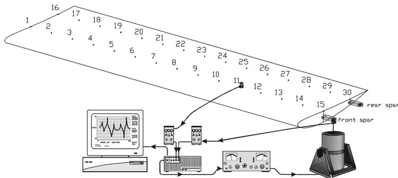
Figure 4. Test set-up wing excitation/response locations.
