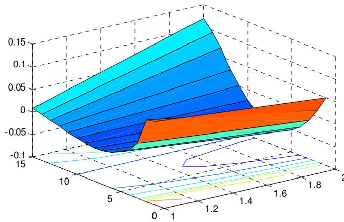
Figure 6. First bending mode identified by the ERA – 45.6 Hz.
