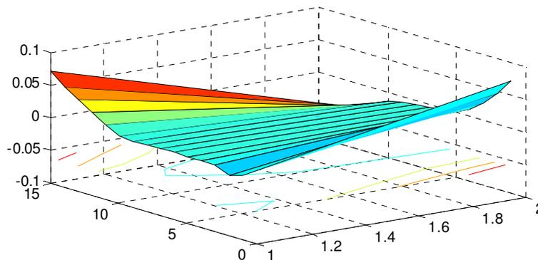
Figure 7. First torsional mode identified by the ERA – 58.2 Hz.
