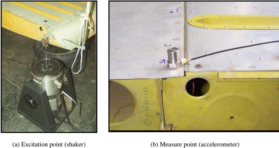
Figure 3. Excitation and measurement devices.
