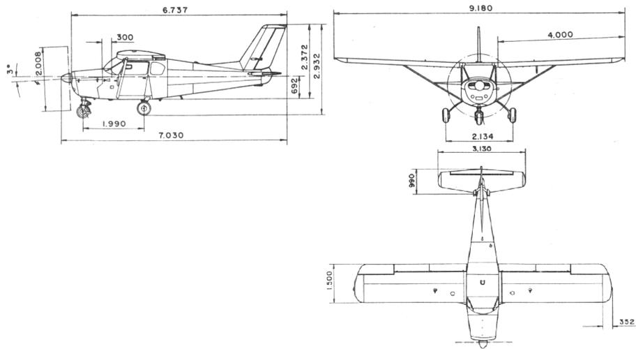
Figure 1. Neiva Regente aircraft (dimensions in meters).
