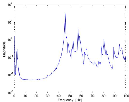
Figure 5. Average Power Spectrum (APS) of 60 measured FRFs.
