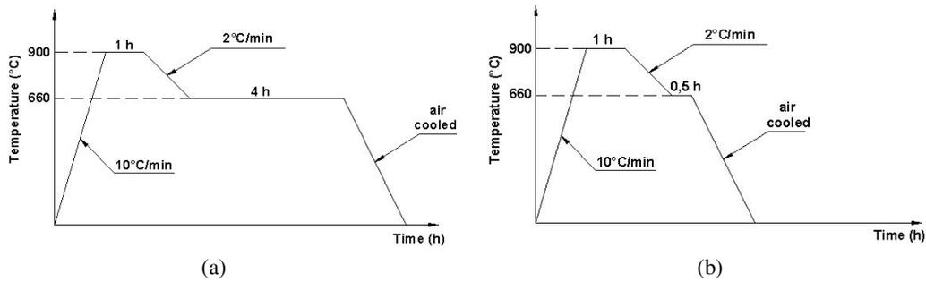
Figure 1. Heat treatment conditions to billet annealing.
