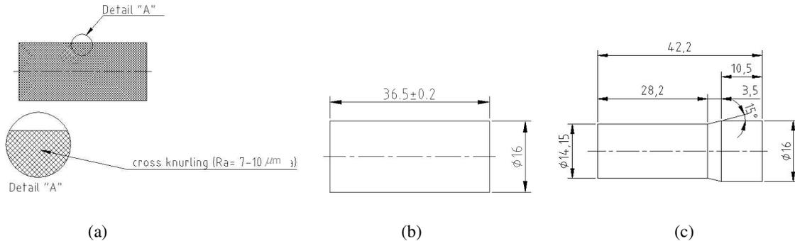
Figure 2. (a) Billet knurled surface, (b) billet dimensions, (c) extruded dimensions.
