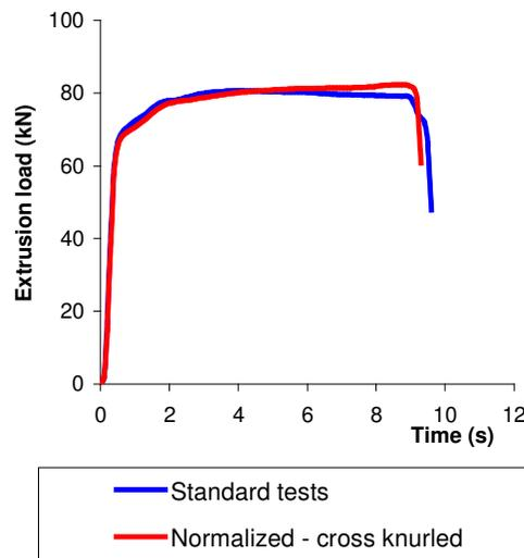
Figure 5. Extrusion load versus process time – lubricant powder soap versus standard conditions.
