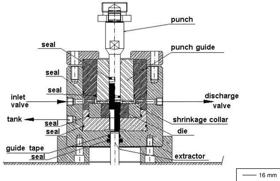
Figure 3. Experimental set up of the extrusion tooling.
