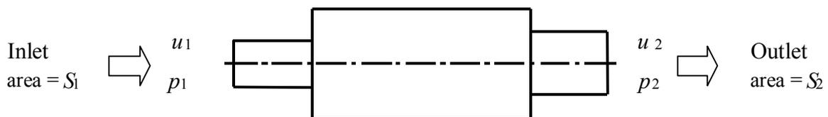
Figure 2- References for expansion chamber.
