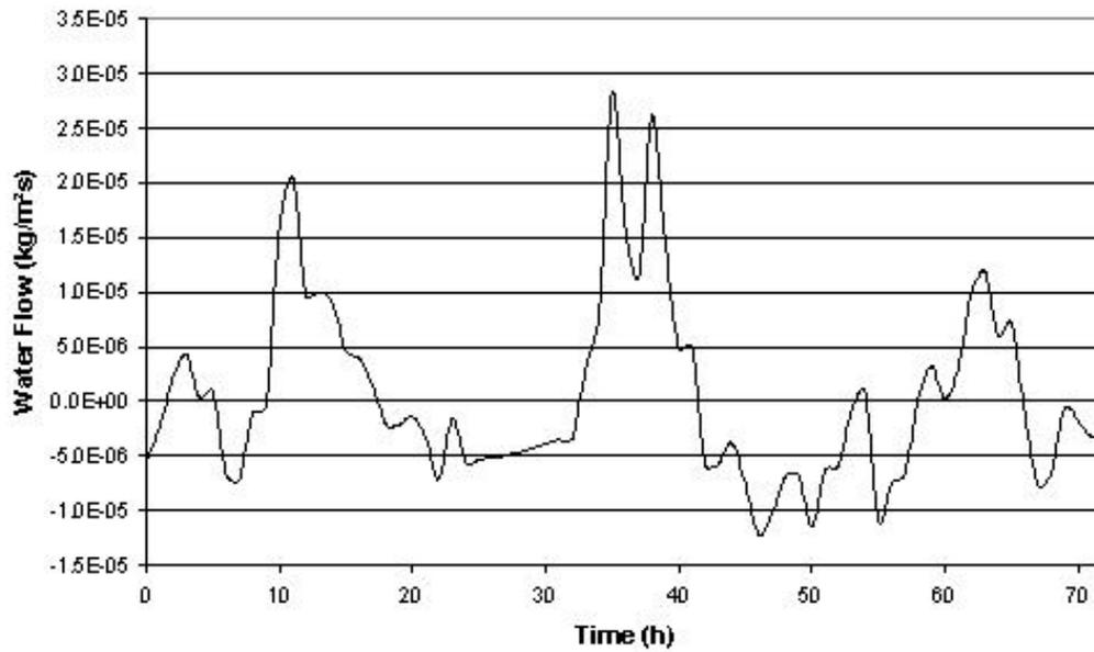
Figure 3. Water vapor flow at the soil surface within the period of 1<sup>st</sup> to 3<sup>rd</sup> of July.
