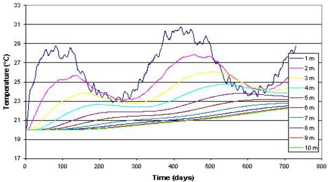
Figure 4. Daily average temperature profiles of the backfill soil for a period of 2 years.
