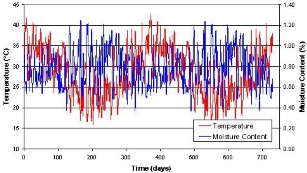
Figure 2. Temperature and moisture content average values at the soil surface for a period of 2 years.
