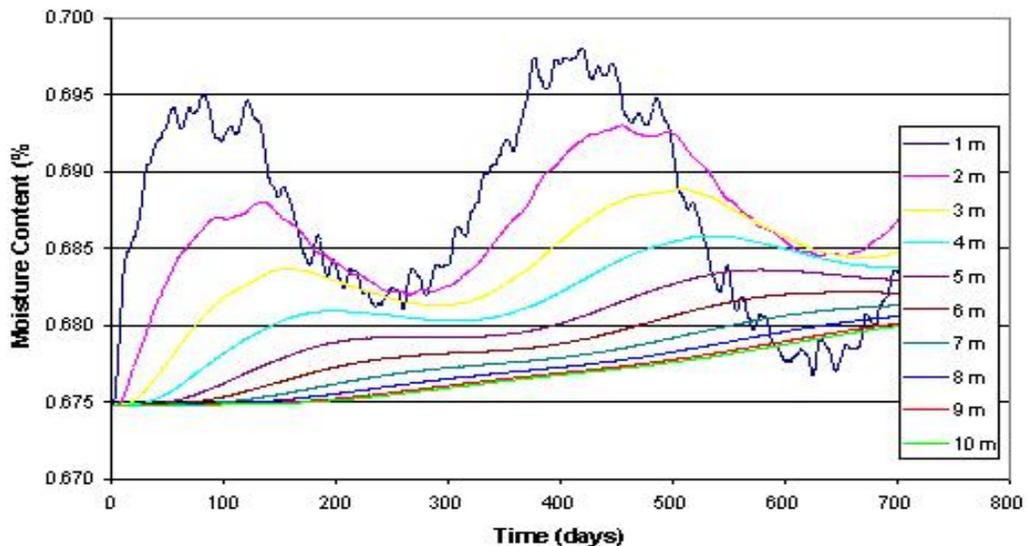
Figure 5. Daily average moisture content profiles of the backfill soil for a period of 2 years.
