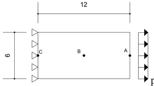
Figure 1. Rectangular bar subjected to Heaviside loading: geometry definitions and boundary conditions.
