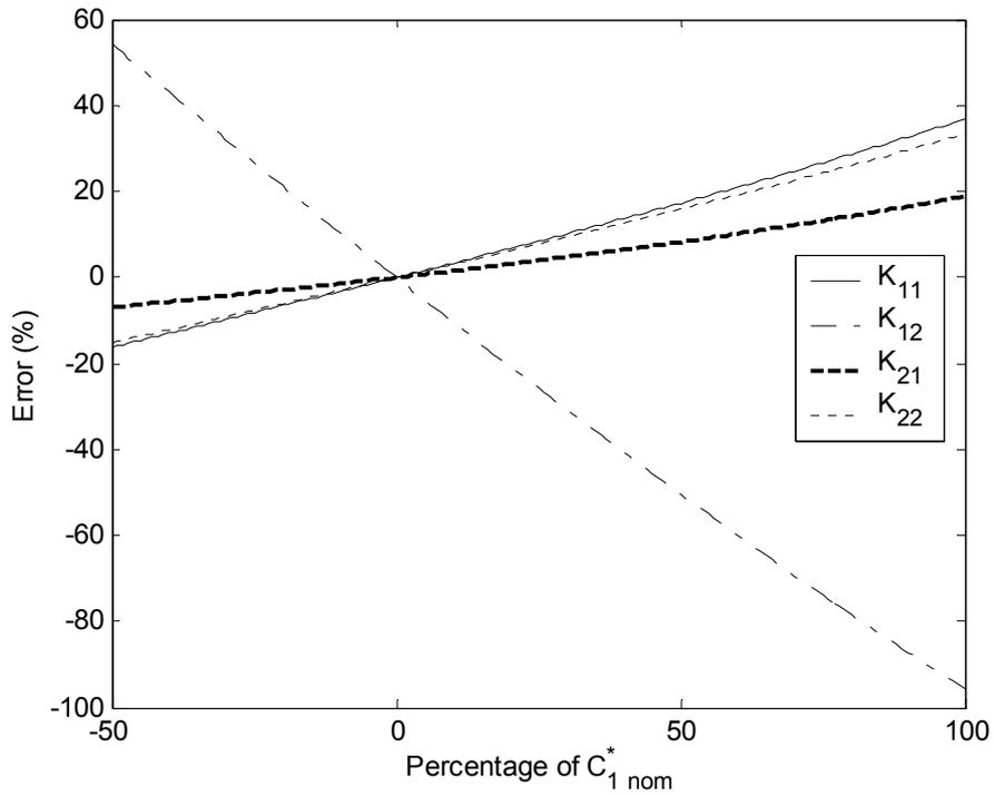
Figure 2. Gain identification errors due to error in  $C_1$ .
