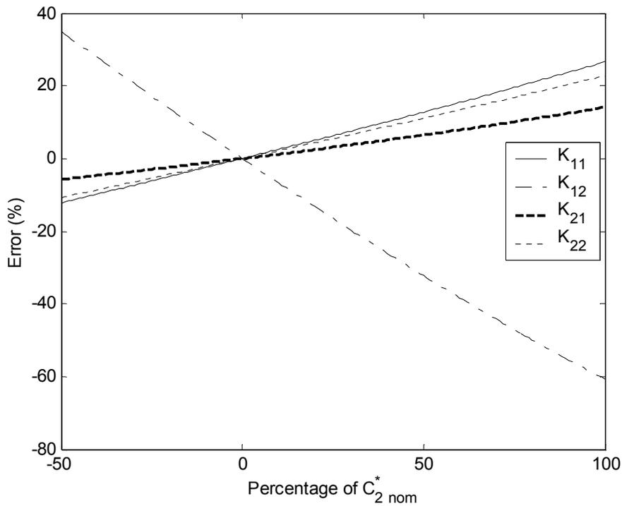
Figure 3. Gain identification errors due to error in  $C_2$ .
