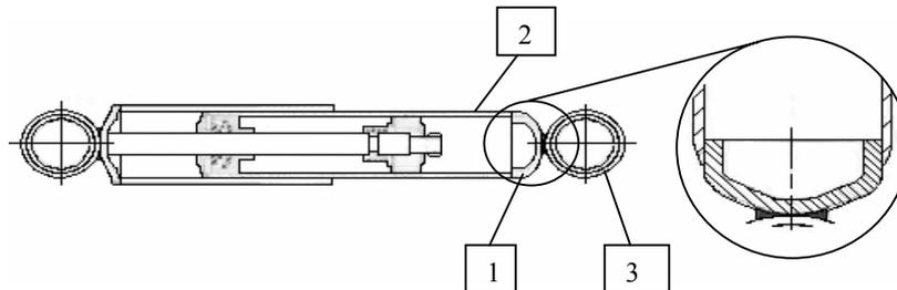
Figure 1. An automotive shock absorber and a detail of the evaluated part.
