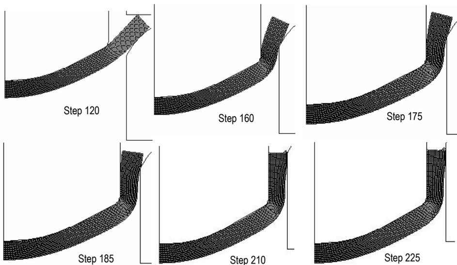
Figure 8. Changes in blank thickness caused by the simulation CA-0-1
