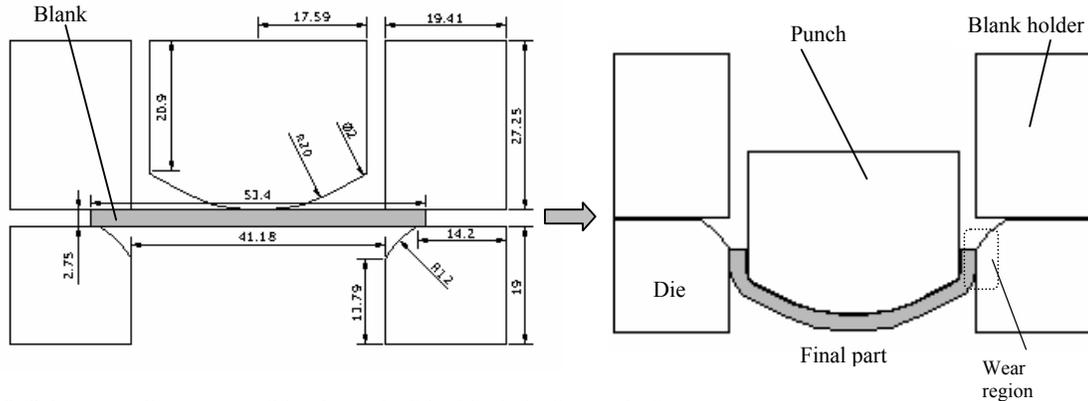
Figure 2. Schematic illustration of the die and of the blank, before and after processing.
