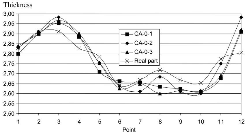
Figure 12. A comparison between the thickness of the real part and of the simulated endcaps.
