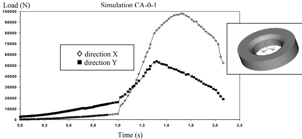
Figure 7. Loads on the die for the simulation CA-0-1
