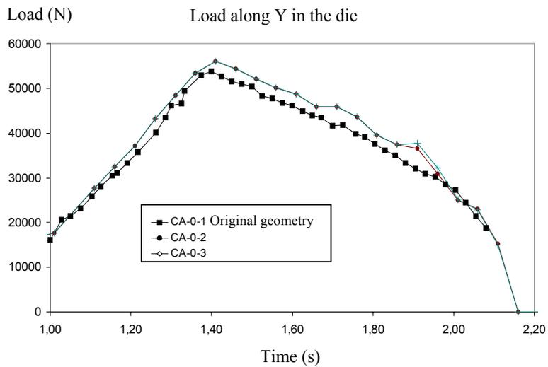
Figure 10. Die loads along the Y direction for the 3 simulations.
