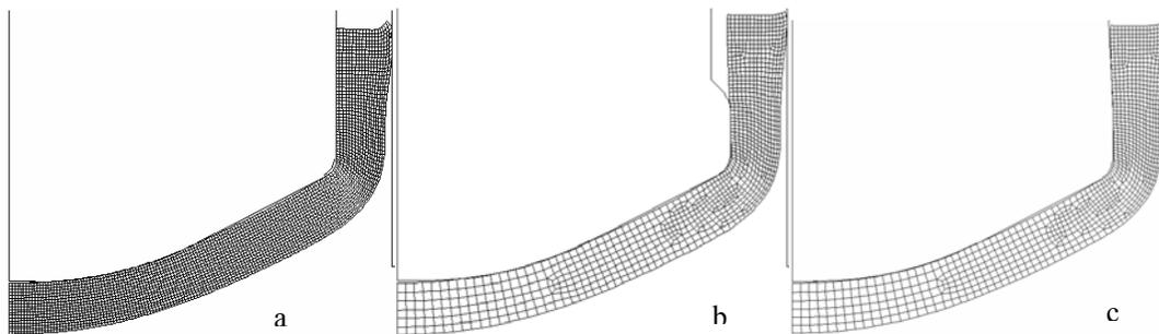
Figure 6. Finite element meshes at step number 225, for simulations CA-0-1 (a), CA-0-2 (b) e CA-0-3 (c)
