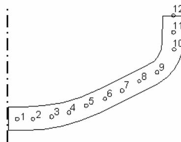
Figure 11. Points along the endcap where the thickness was measured for the real part and for the simulations.
