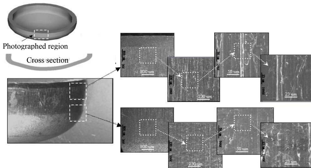
Figure 3. Details of the scratched regions in the shock absorber endcap.
