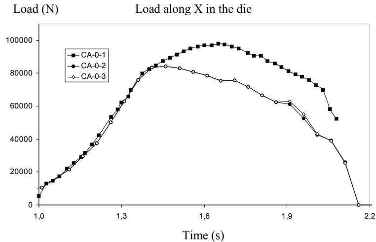
Figure 9. Die loads along the X direction for the 3 simulations.
