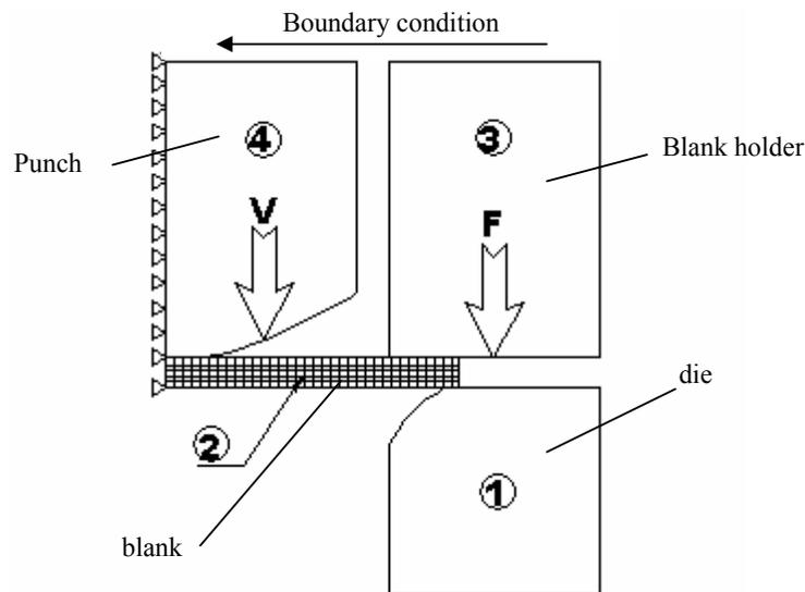
Figure 4. Illustration of the dies used in the DEFORM program, including the employed boundary conditions.
