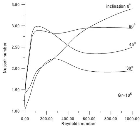
Figure 11. Average normalized Nusselt number in function of Reynolds number for various inclinations and  $Gr=10^5$ .
