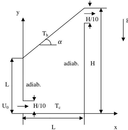
Figure 1. The vented enclosure and the coordinate system
