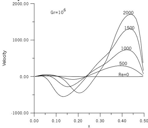
Figure 7. Vertical components of the velocity along the middle horizontal line for values of the Reynolds number.
