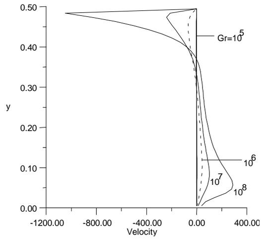
Figure 7. Horizontal velocity component profile along the middle vertical line of the cavity.
