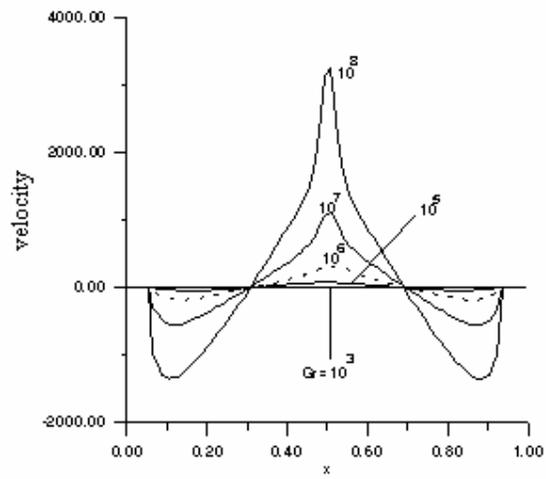
Figure 8. Vertical velocity component profile along the middle horizontal line of the cavity.
