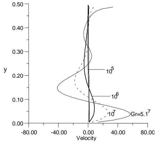
Figure 3. Horizontal velocity component profile along the middle vertical line of the cavity.
