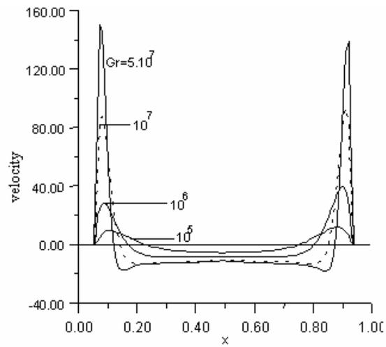
Figure 4. Vertical velocity component profile along the middle horizontal line of the cavity.
