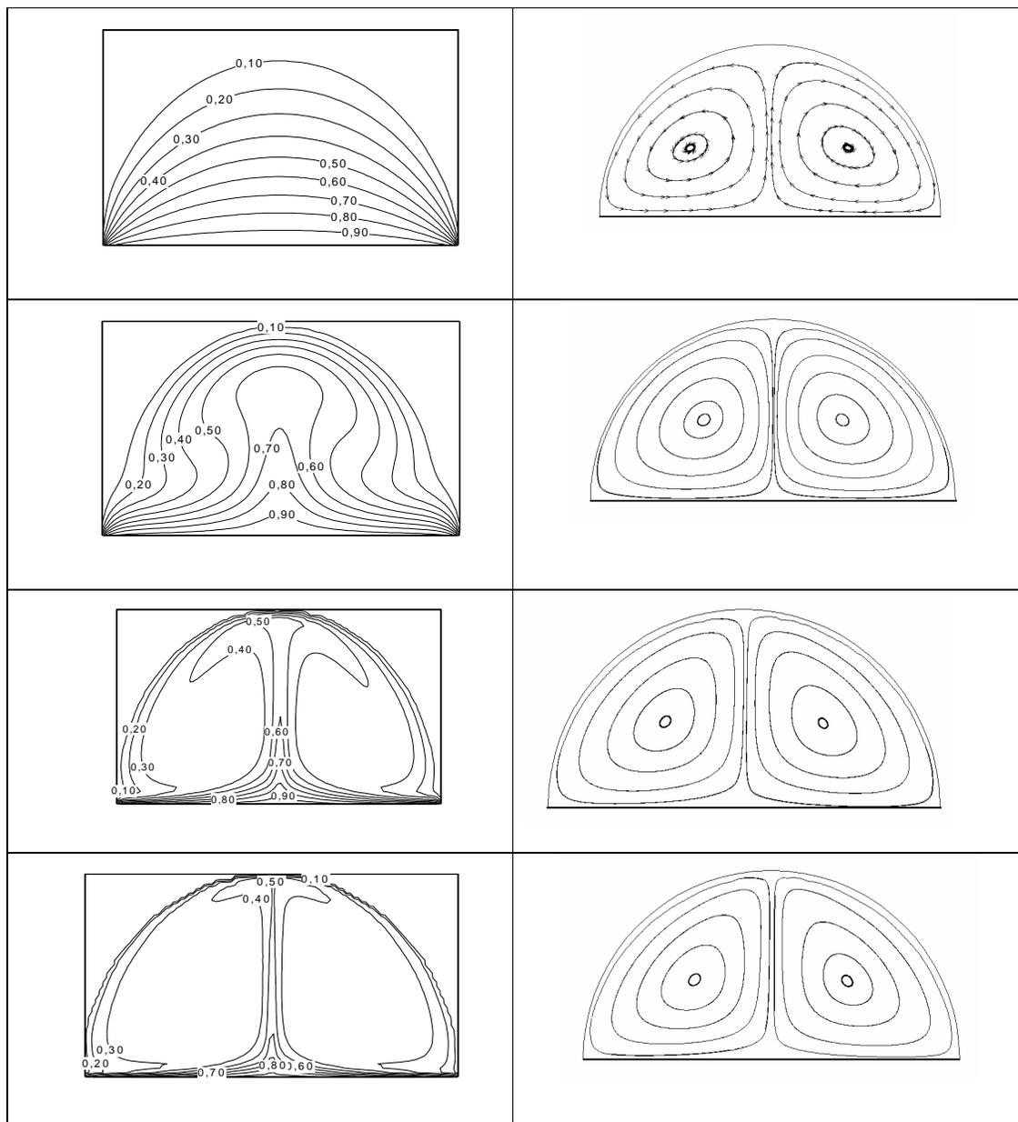
Figure 6. Isotherms (left) and streamlines (right) for the steady state flow for  $Gr = 1.0 \times 10^3$ ,  $Gr = 1.0 \times 10^5$ ,  $Gr = 1.0 \times 10^7$ ,  $Gr = 1.0 \times 10^8$ .
