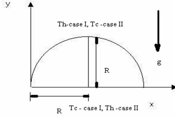
Figure 1: Semi-cylindrical cavity and the coordinate system.
