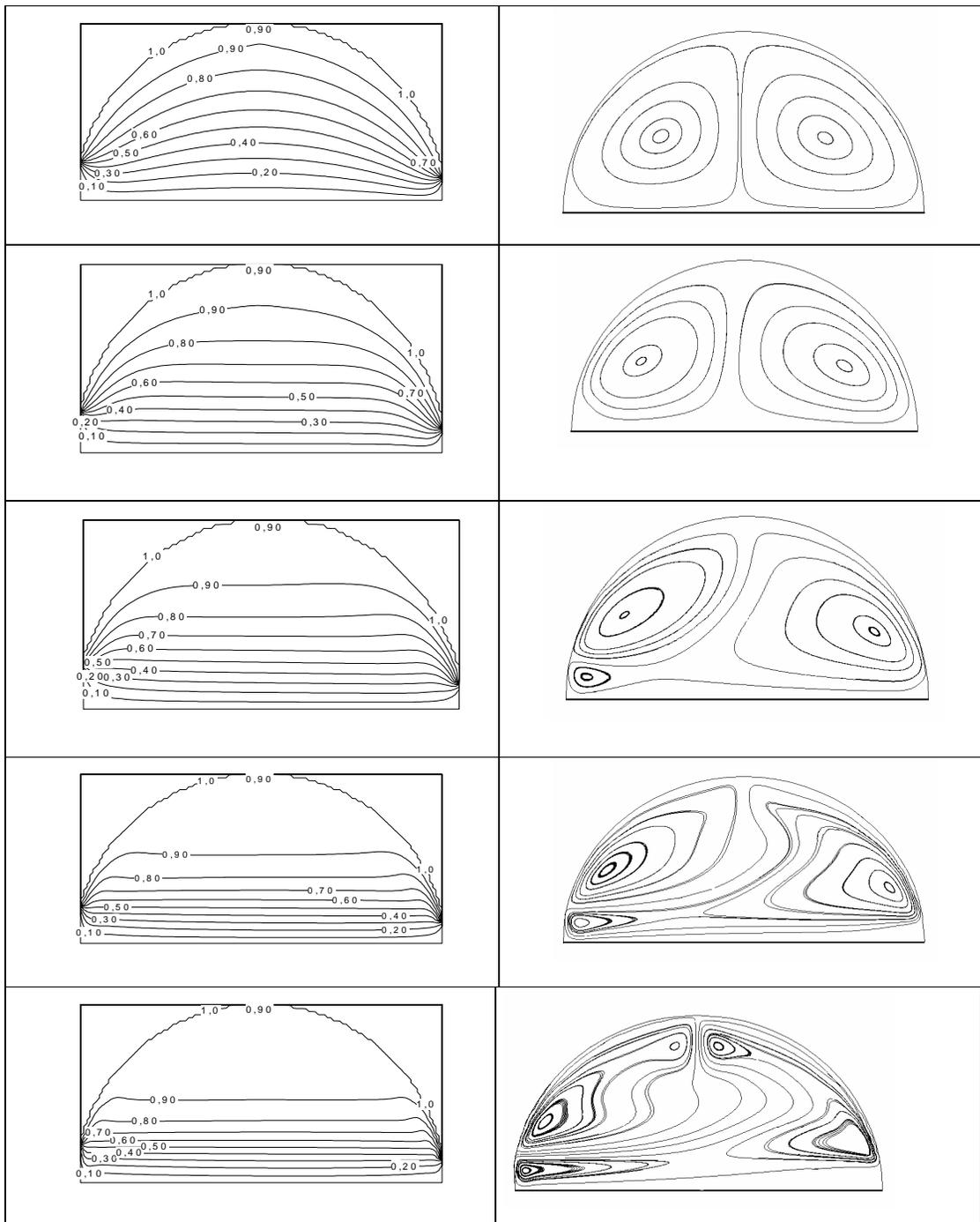
Figure 2. Isotherms (left) and streamlines (right) for the steady state flow  $Gr = 1.0 \times 10^3$ ,  $Gr = 1.0 \times 10^5$ ,  $Gr = 1.0 \times 10^6$ ,  $Gr = 1.0 \times 10^7$ ,  $Gr = 5.0 \times 10^7$ .
