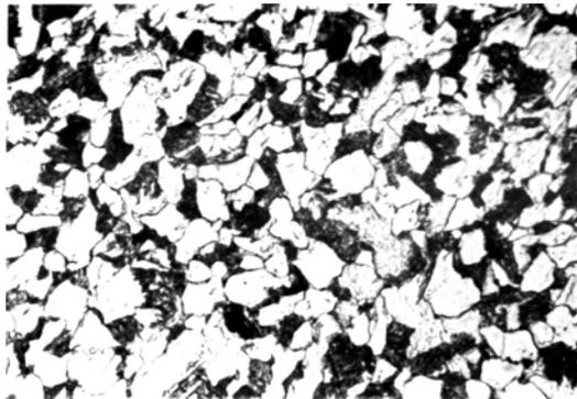
Figure 2. Microstructure of normalised AISI/SAE 8620 steel (500X)
