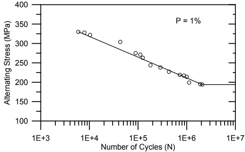
Figure 5. S-N-Fatigue curve of undamaged specimens with failure probability  $P = 1\%$  or reliability  $R = 99\%$
