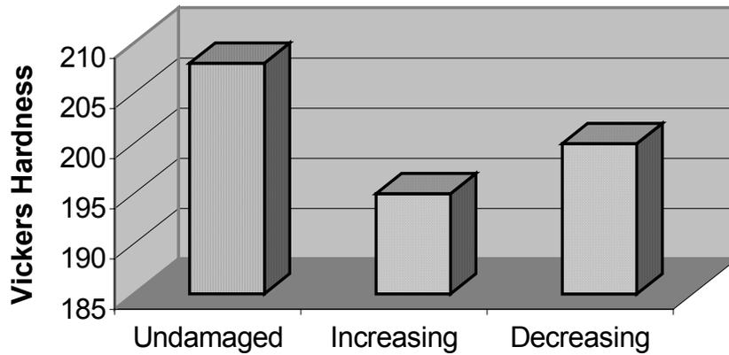
Figure 7. Influence of fatigue damage on Vickers Hardness
