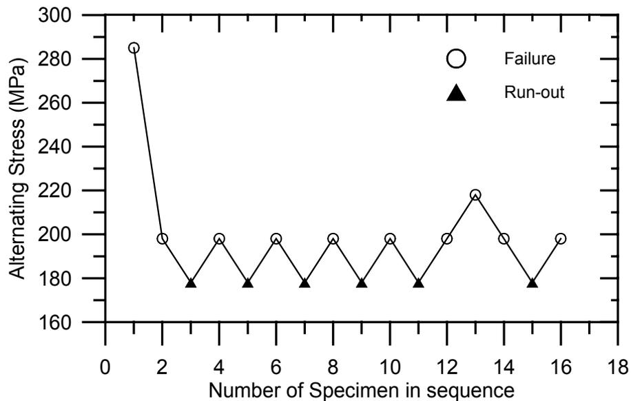
Figure. 4. Up-and-Down Fatigue test of undamaged specimens
