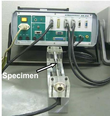
Figure 3. Barkhausen device and clamping fixture for measuring BN
