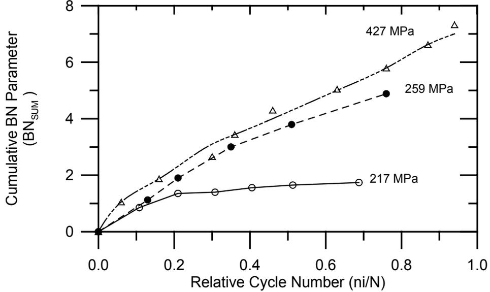
Figure 11. Influence of relative fatigue cycle on cumulative BN parameter
