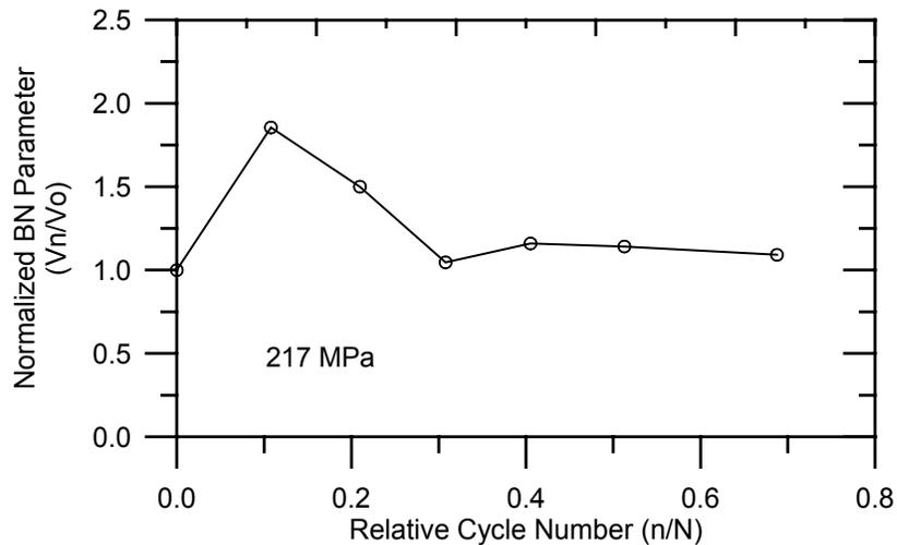
Figure 10. Influence of relative fatigue cycle on normalized Barkhausen noise RMS values
