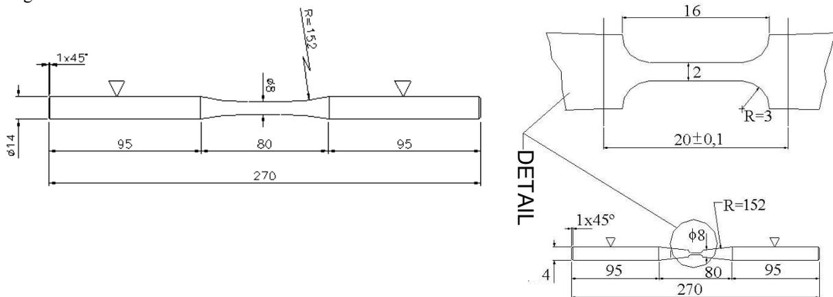
Figure 1. Fatigue Specimen (Dimensions in mm) – Rotating-bending for step-stress fatigue test (left); Axial for Barkhausen measurements (right)
