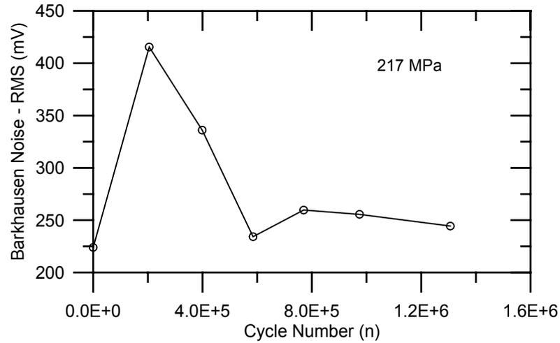
Figure 9. Changes in Barkhausen noise RMS values with number of fatigue cycles
