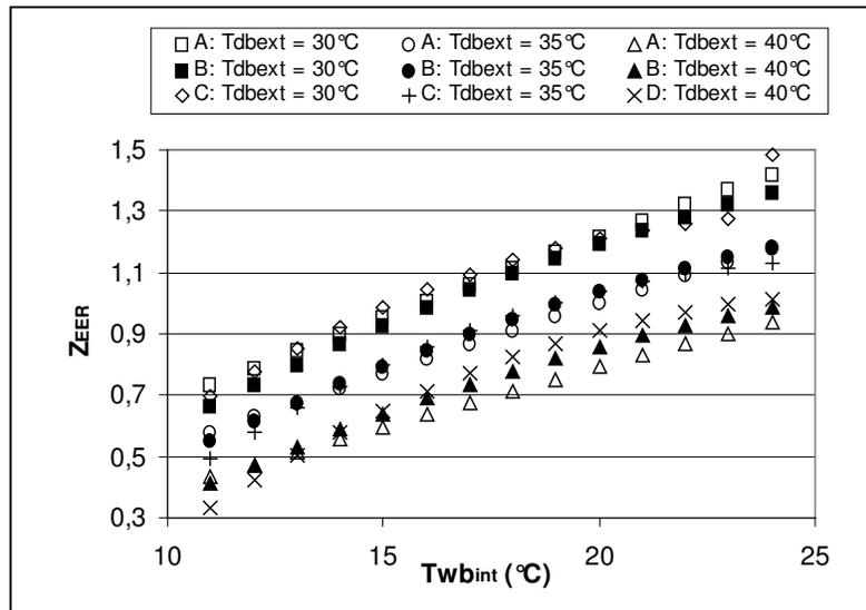
Figure 4. EER factor comparison under several room-side and outdoor-side temperature conditions.
