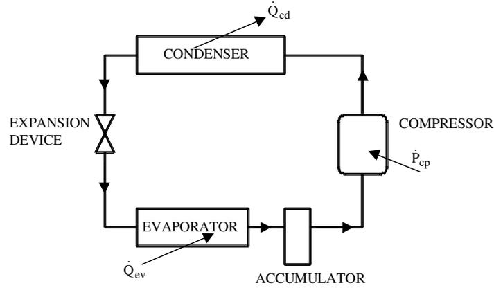
Figure 1. Vapor-compression cycle.
