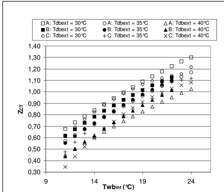
Figure 3. Comparative of total cooling capacity factor under several room-side and outdoor-side temperature conditions.
