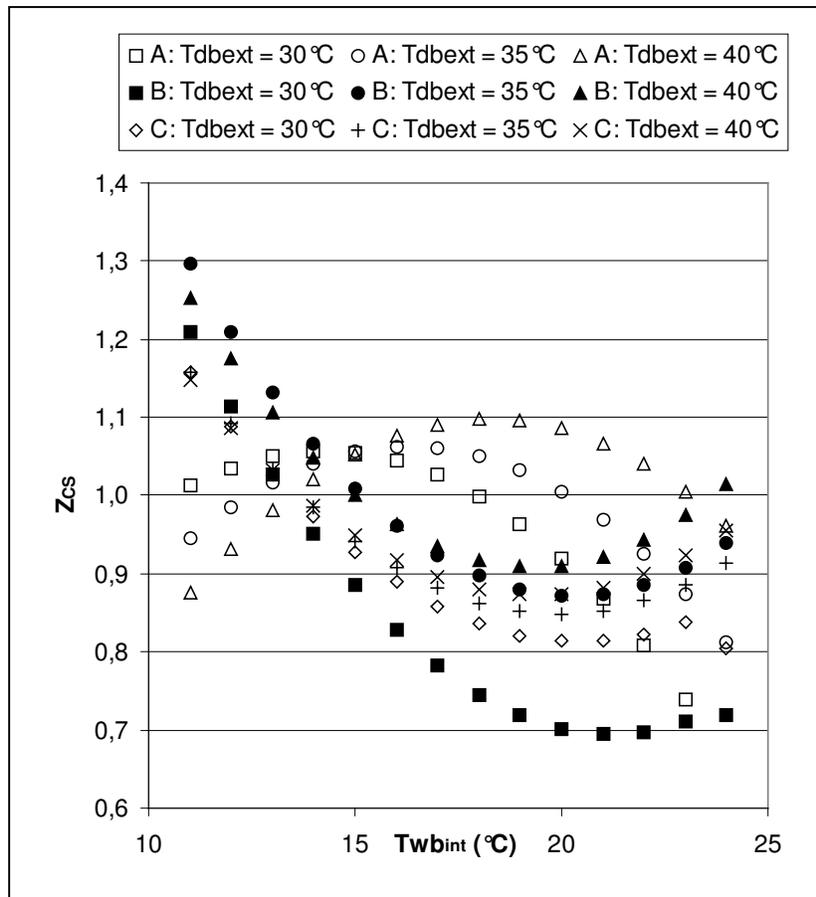
Figure 5. Comparative of sensible capacity under several room-side and outdoor-side conditions.
