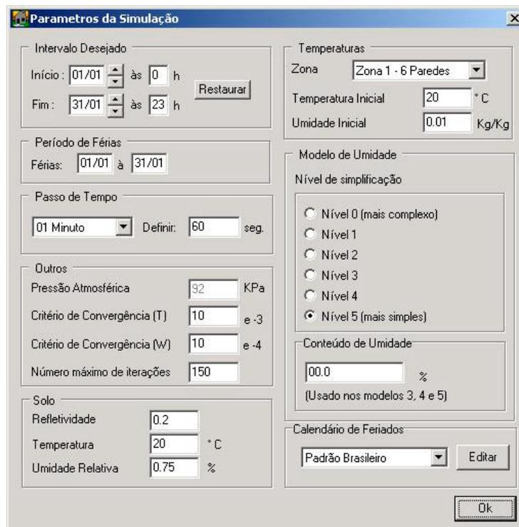
Figure 9: Program Domus input parameters for simulating the single-zone building .
