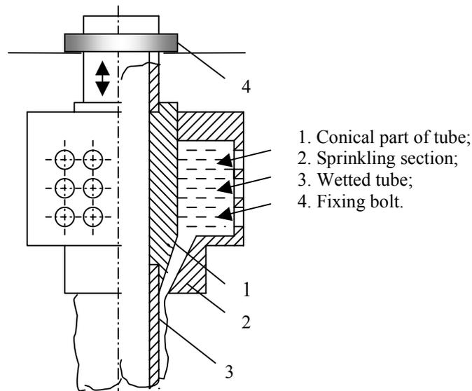
Figure 3. Distribution device for generation of liquid film flow on vertical tubes.
