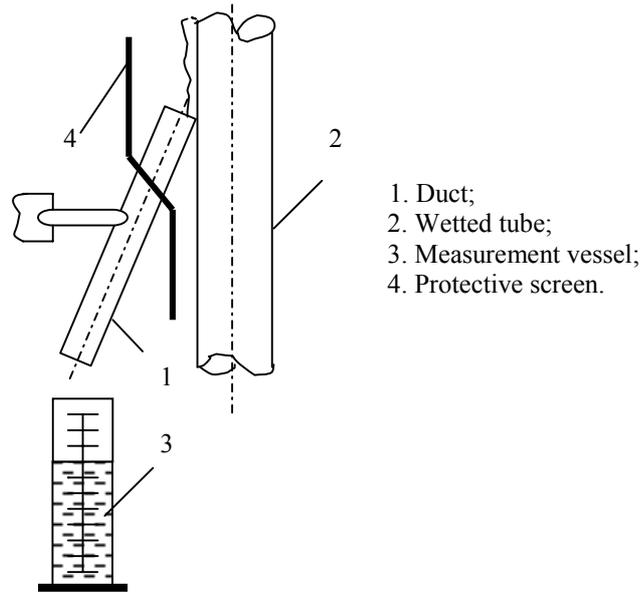
Figure 4. Construction of control device.
