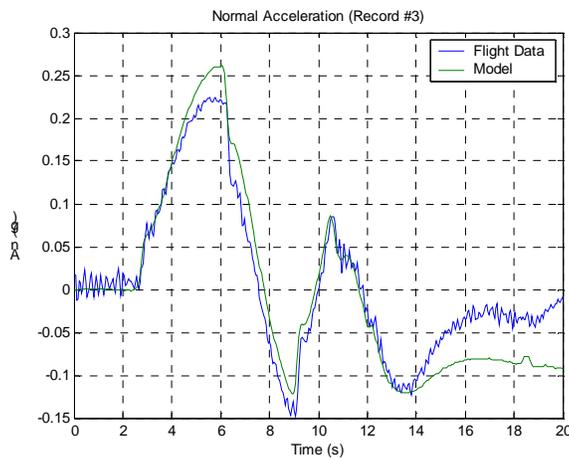
Figure (5) – Model and aircraft acceleration responses.
