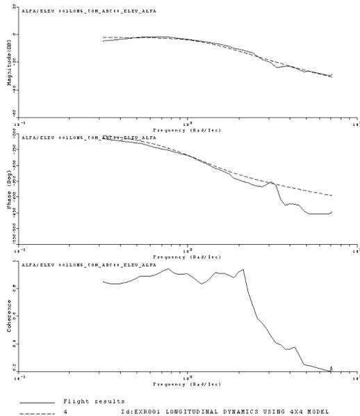
Figure (6) – Angle of attack FRF matching.
