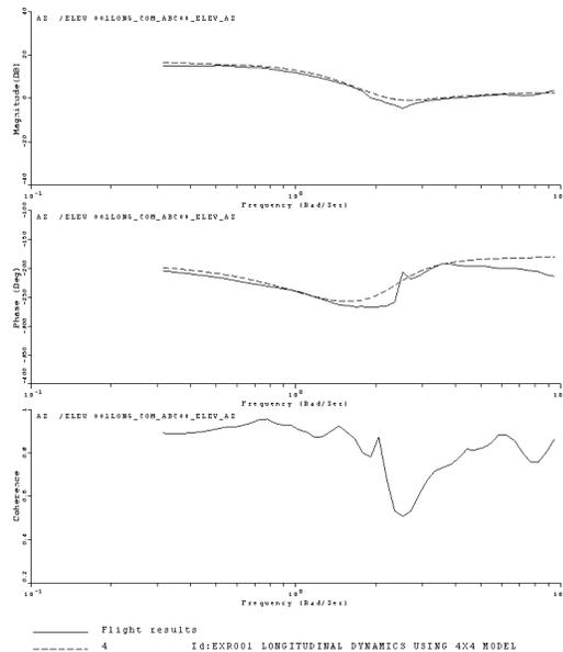
Figure (9) – Acceleration FRF matching.
