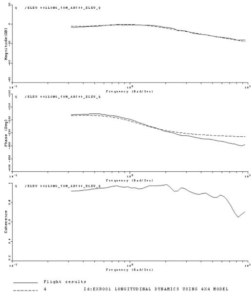
Figure (7) – Pitch rate FRF matching.
