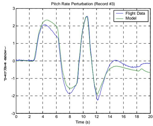
Figure (3) – Model and aircraft angle of attack responses. Figure (4) – Model and aircraft pitch rate responses.
