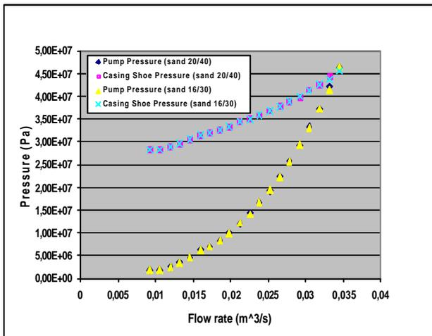
Figure 8. Effect of particle size on pump and casing shoe pressures.
