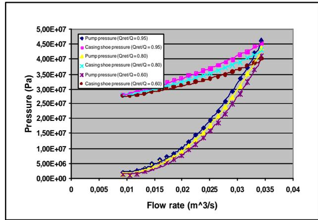
Figure 11. Effect of return rate on pump and casing shoe pressures.
