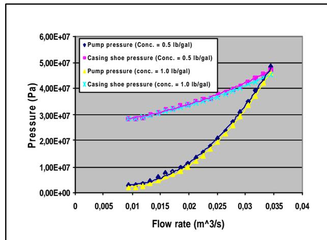
Figure 9. Effect of particle concentration on pump and casing shoe pressures.
