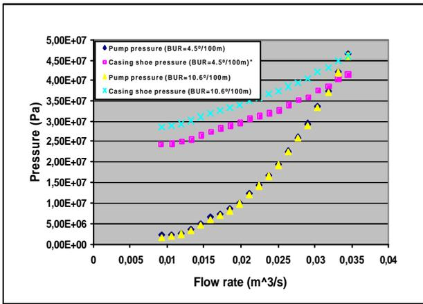
Figure 10. Effect of well path on pump and casing shoe pressures.
