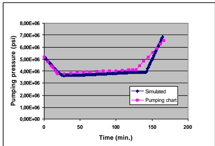
Figure 12. Comparison of the results obtained by the numerical simulator with the pressures registered during the operation.
