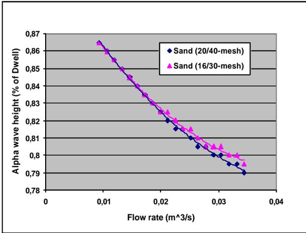
Figure 6. Effect of particle size on alpha wave height.
