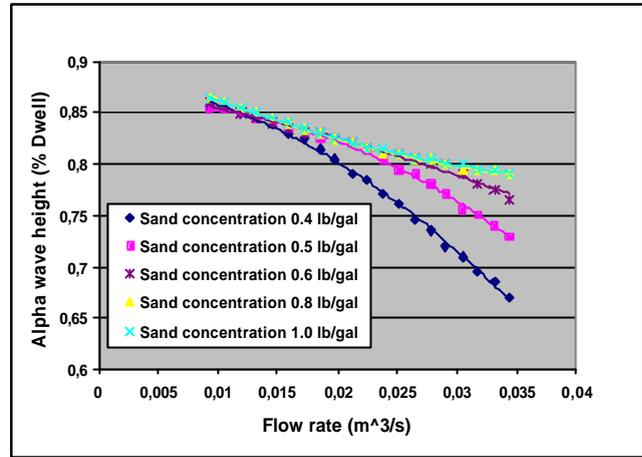
Figure 7. Effect of particle concentration on alpha wave height.
