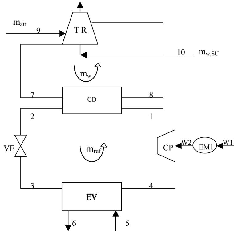
Figure 1. Refrigeration cycle by compression.
