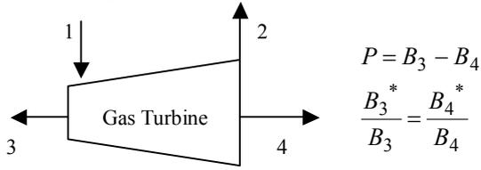
Figure 3. Unitary exergetic costs to fuel flows in a gas turbine.
