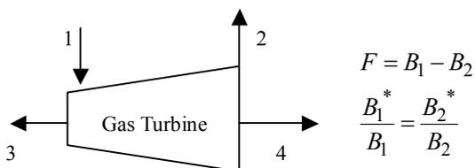
Figure 2. Unitary exergetic costs to fuel flows in a gas turbine.
