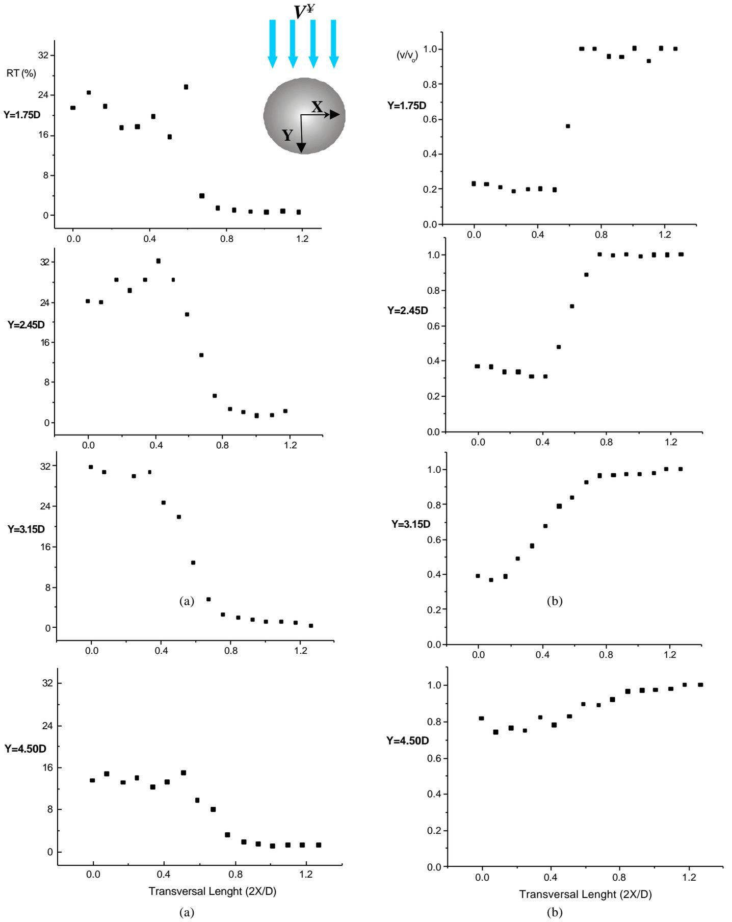
Figure 8. Relative turbulence level (a) and velocity profiles (b) as function of the transversal length, for Reynolds number 3000.
