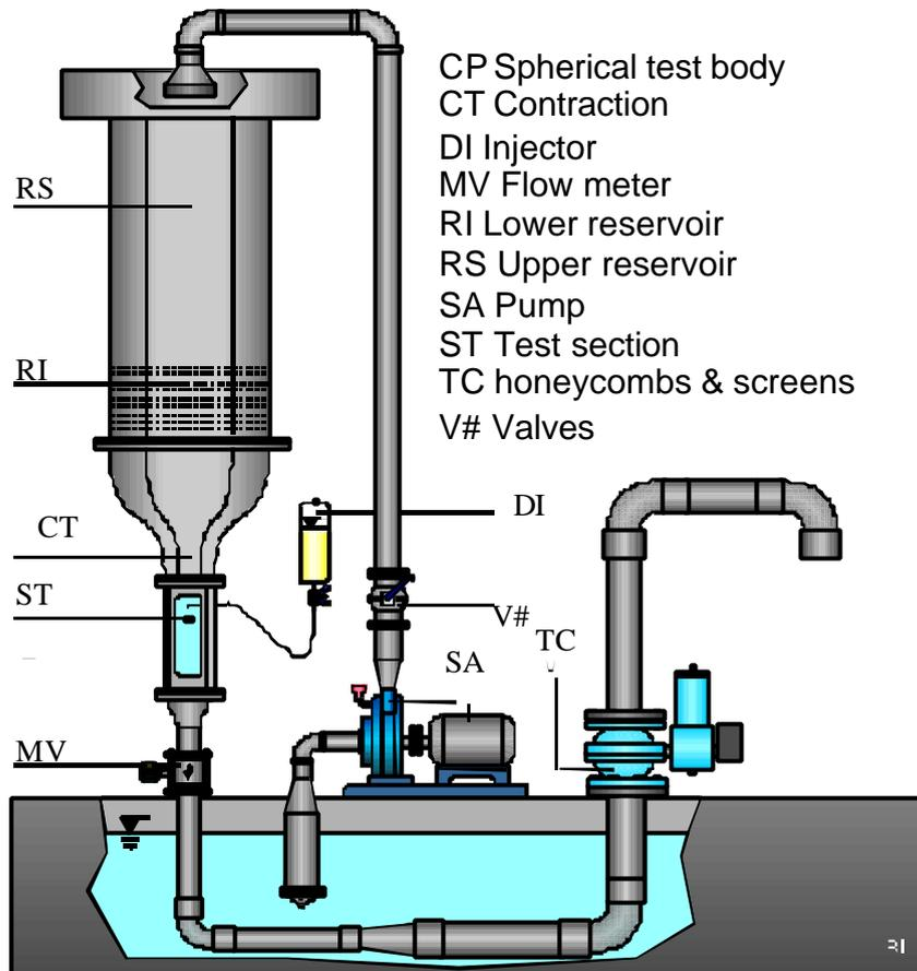
Figure 1. The low-turbulence vertical hydrodynamic tunnel.
