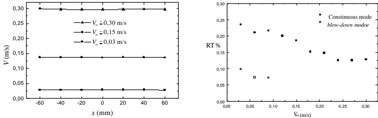
Figure 2. Free stream velocity profile and relative turbulence intensity in the test section of the tunnel.
