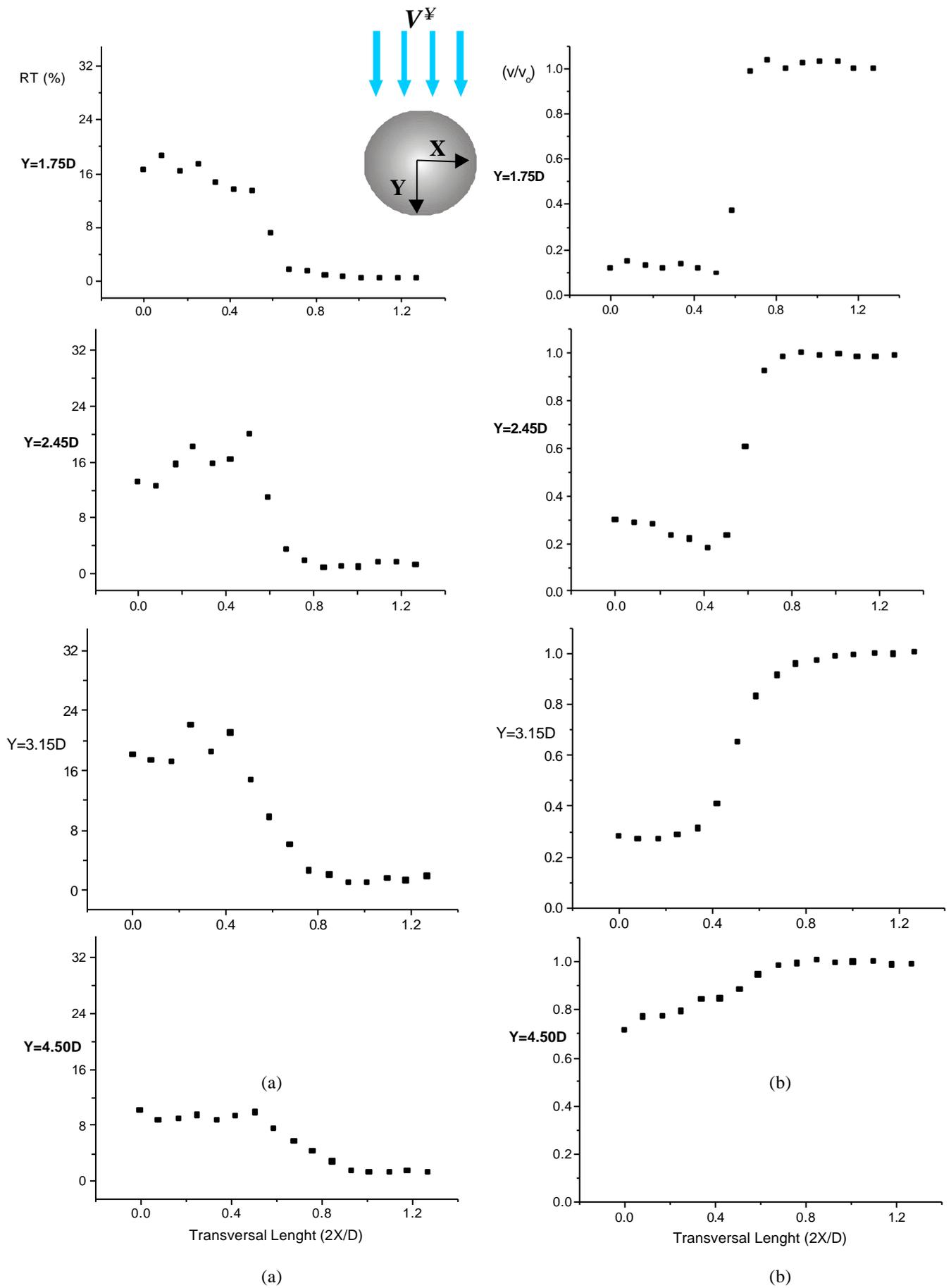
Figure 7. Relative turbulence level (a) and velocity profiles (b) as function of the transversal length, for Reynolds number 2000.
