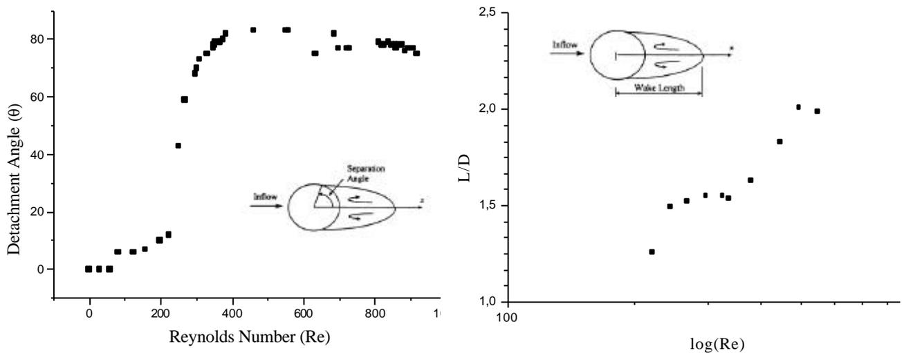
Figure 5. Detachment angle ( $\theta$ ) and length bubble recirculating ( $L$ ) in function of Reynolds number
