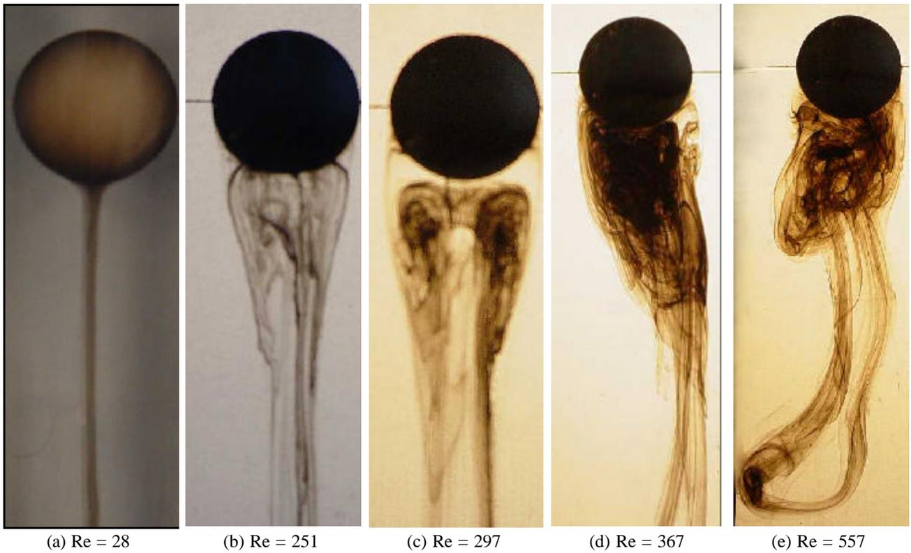
Figure. 4 sphere wake visualized images in close view.
