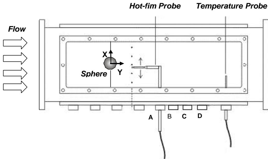
Figure 3 Experimental assemble utilized in the test section.
