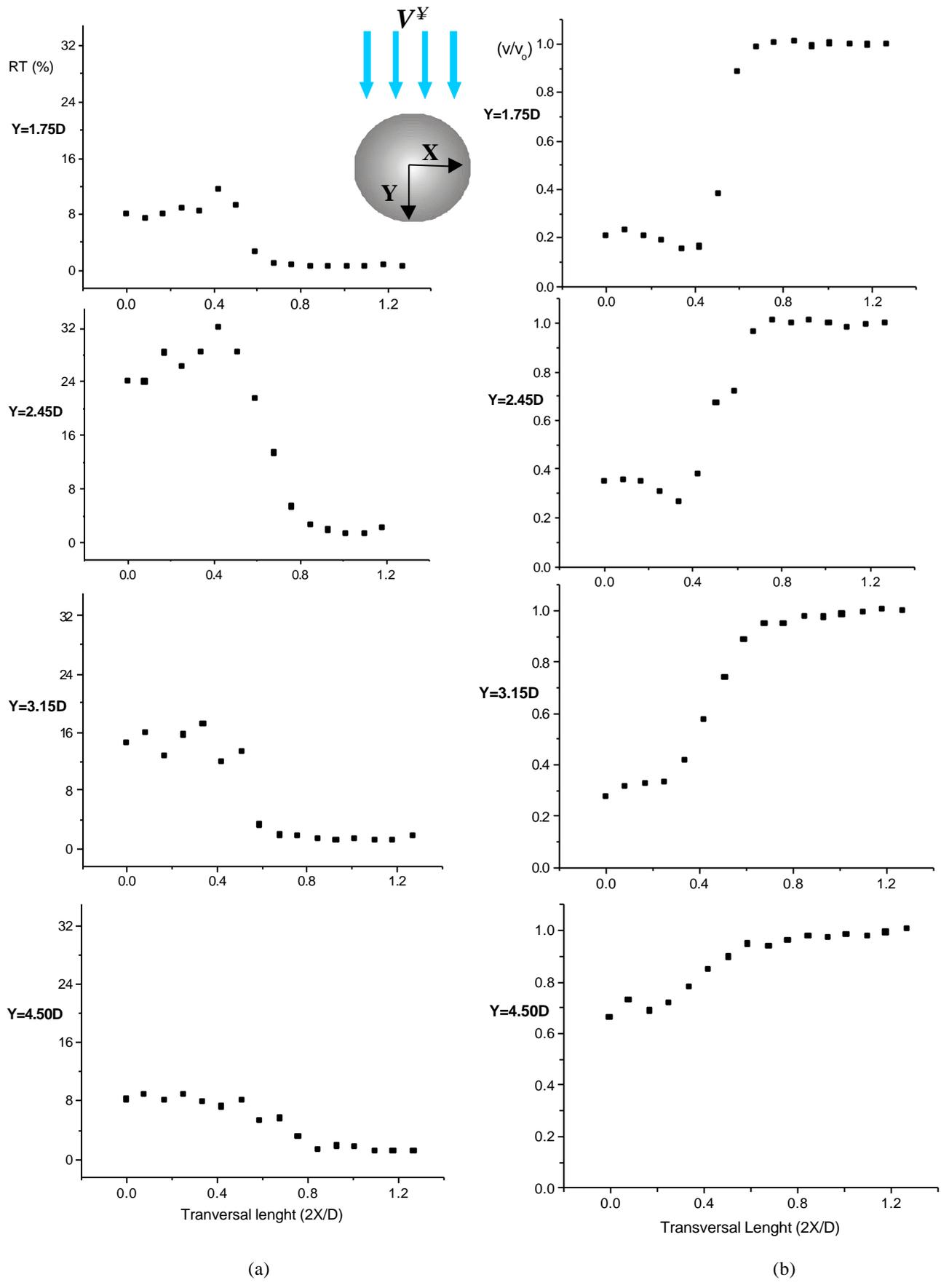
Figure 6. Relative turbulence level (a) and velocity profiles (b) as function of the transversal length, for Reynolds number 1000.
