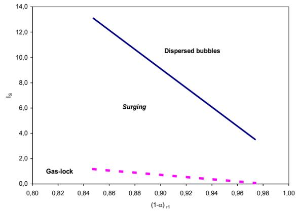
Figure 7. Mapping of the flow regime inside the impeller
