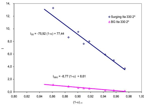
Figure 6. Onset of surging and gas-lock conditions
