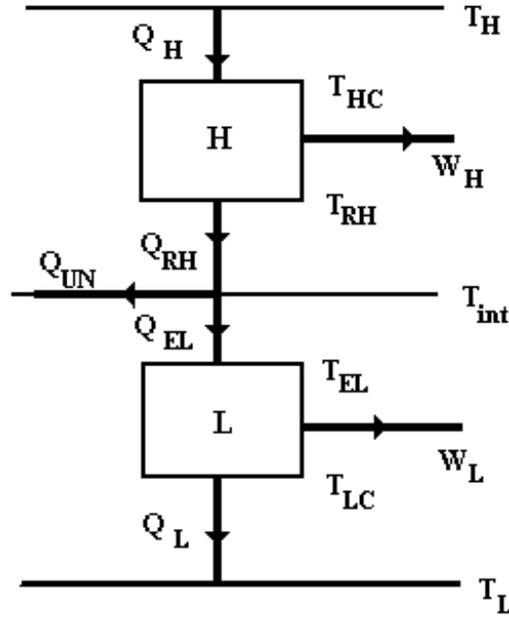
Figure 2. Series combined cycle with intermediate heat losses. Maximization of work output.
