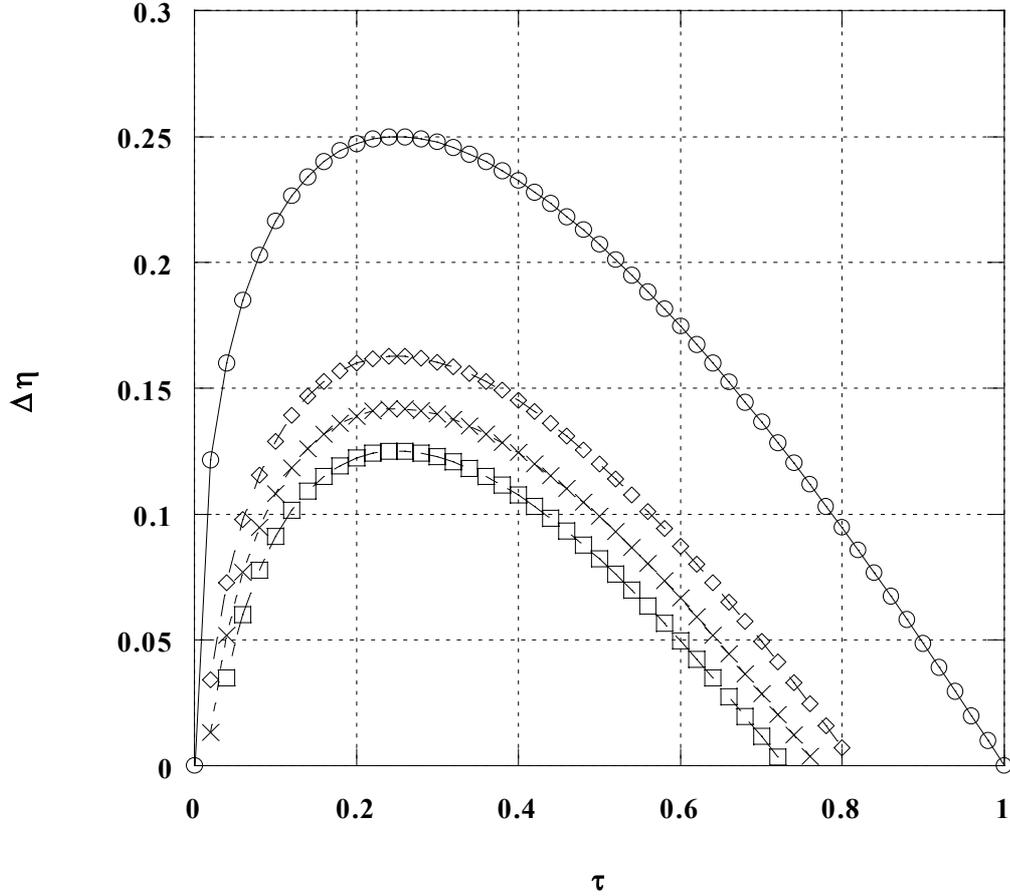
Figure 3. Reduction of the series combined cycle thermal efficiency for the maximization of work output. Symbol  $\circ$  refers to Eq. (14), Other symbols refer to Eq. (30):  $\square$  is for  $\tau_{\text{int}} = 0.6$  ,  $\times$  for  $\tau_{\text{int}} = 0.1$  and  $\square$  for  $\tau_{\text{int}} = 0.25$  .
