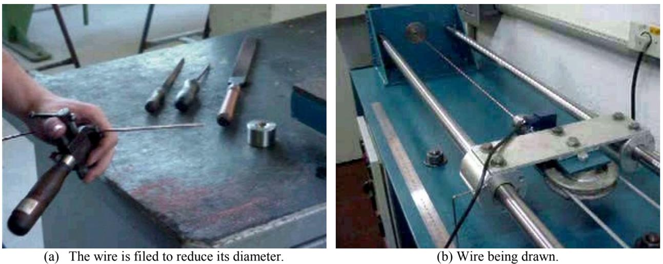
Figure 4. Illustration showing the preparation of the wire for drawing.
