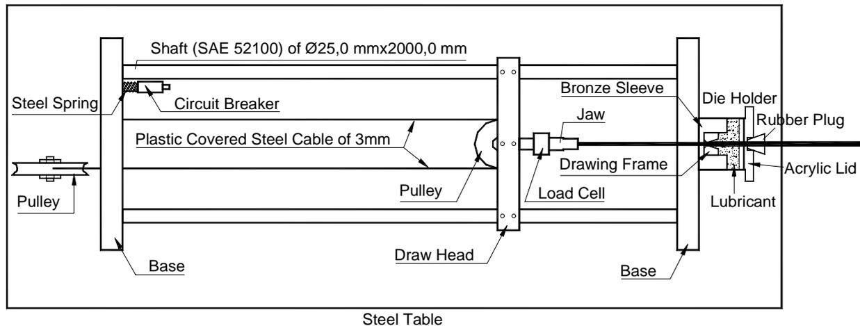
Figure 2. Schematic diagram showing plan view of the present wire drawing machine.
