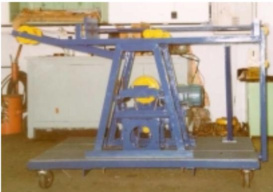
1. Prototype wire drawing machine.
