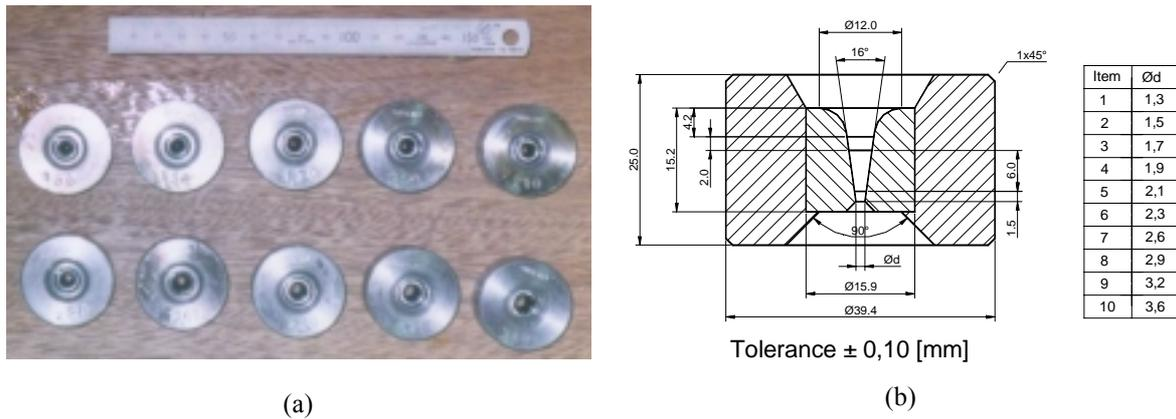
Figure 3. Tungsten-carbide dies for wire drawing (a); and a cross section of the die showing the tungsten-carbide die cased with the SAE 1040 steel (b).
