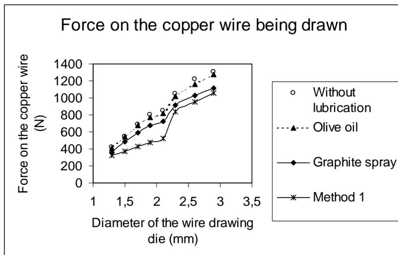
Figure 6. Variation achieved of the wire drawing forces for copper wire.
