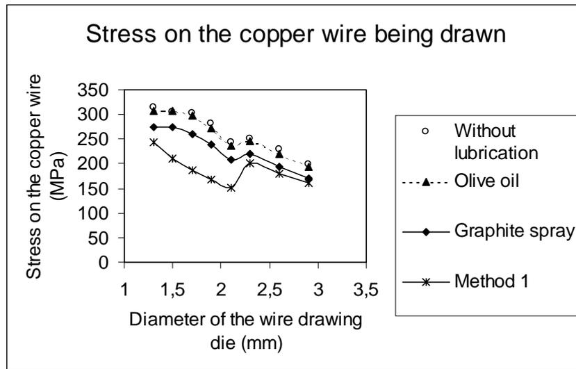
Figure 7. Variation achieved of wire drawing stresses for copper wire.
