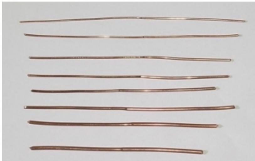
Figure 8. Variation of the diameter of the copper wire obtained from the wire drawing process. The wire starts with diameter of 3.2mm and ends with a final drawing frame diameter of 1.3mm.
