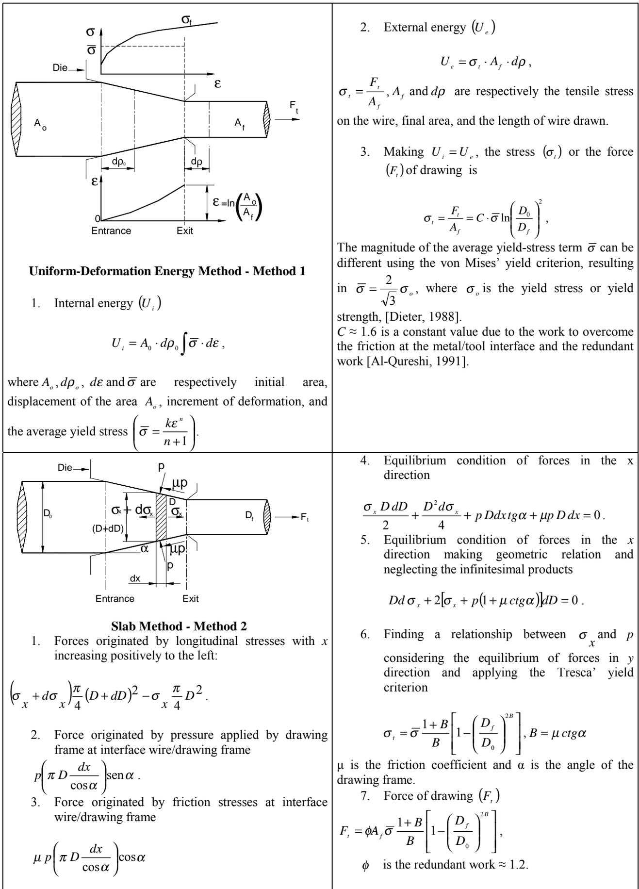
Figure 5. Schematic drawing of the geometry and the stresses involved in the drawing processing by the Uniform-Deformation Energy (Method 1) and Slab (Method 2) methods.
