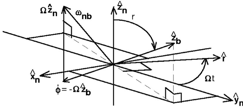
Figure 2- Classic coning motion: spin axis  $\hat{z}_b$  precesses with rate  $\Omega$  about precession axis  $\hat{z}_n$ , maintains constant cone half-angle angle  $r$ , and body spin rate  $\dot{\phi} = -\Omega$  about spin axis.
