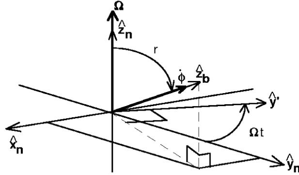
Figure 1 - Coning motion: body spins with rate  $\dot{\phi}$  about its spin axis  $\hat{z}_b$ , which simultaneously precesses with rate  $\Omega$  about precession axis  $\hat{z}_n$ .
