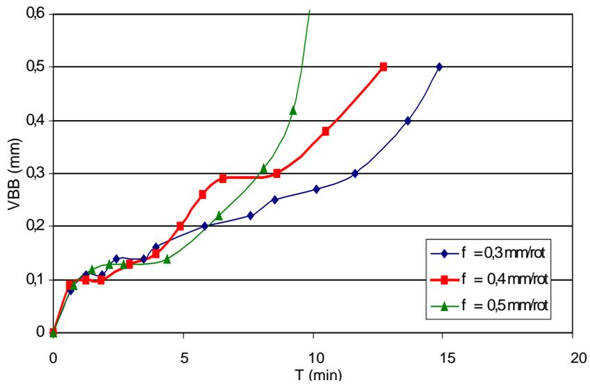
Figure 3. Tool wear against cutting time for the VRA tool ( $v_c=200$  m/min and  $a_p=1$ mm).
