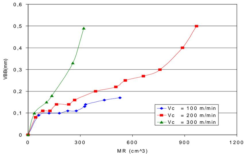
Figure 2. Tool wear against metal removal for the VRA tool ( $f=0,3$  mm/rot e  $a_p=1$ mm).
