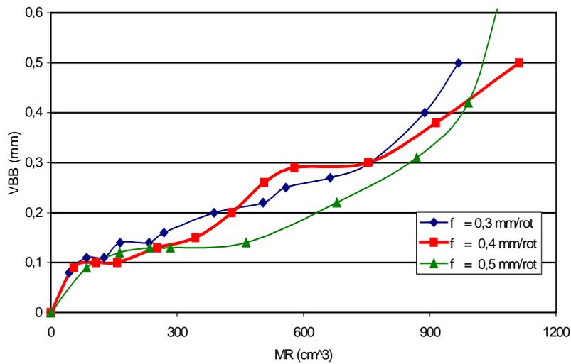
Figure 4. Tool wear against metal removal for the VRA tool ( $v_c=200$  m/min and  $a_p=1$ mm).
