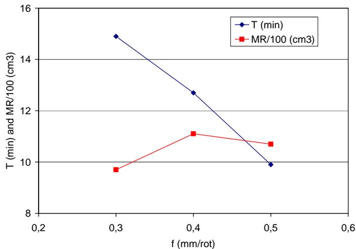
Figure 6. Tool life and metal removal against feed rate for the VRA tool ( $v_c=200\text{m/min}$  and  $a_p=1\text{mm}$ ).
