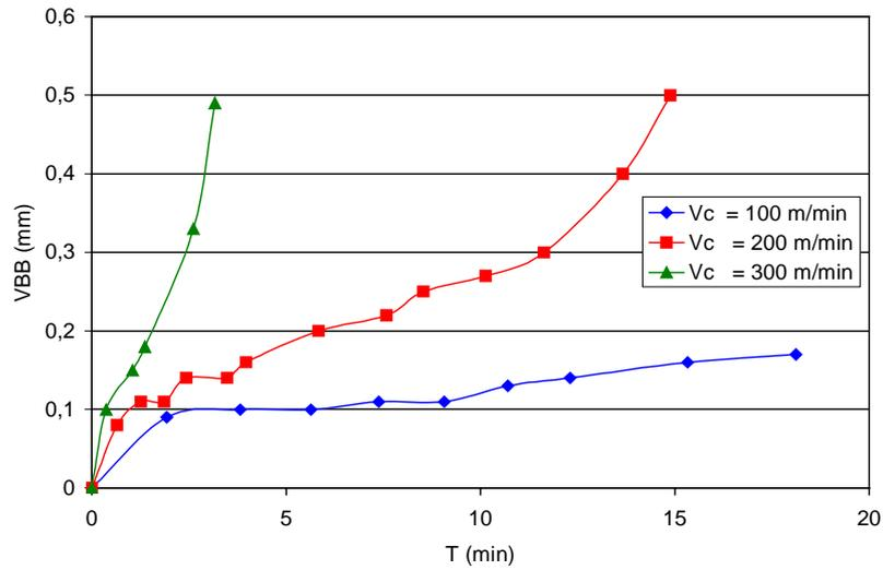
Figure 1. Tool wear against cutting time for the VRA tool ( $f=0,3$  mm/rot e  $a_p=1$ mm).
