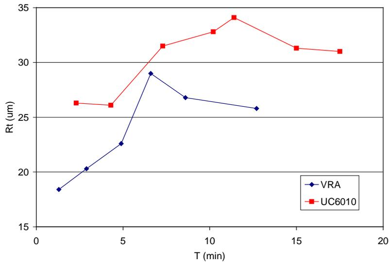
Figure10. Maximum surface roughness (Rt) against cutting time for VRA and UC6010 tools ( $v_c=200$  m/min,  $f=0,4$  mm/rot e  $a_p=1$ mm).
