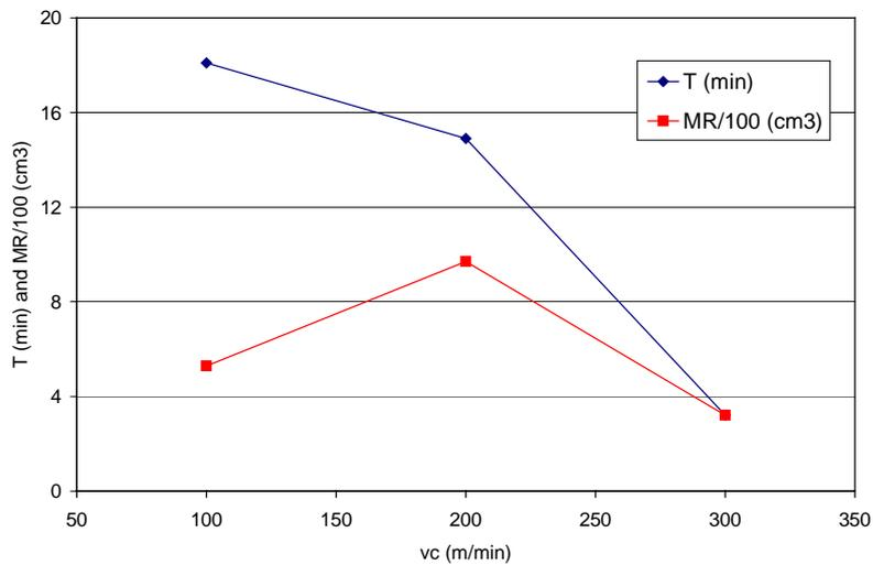
Figure 5. Tool life and metal removal against cutting speed for the VRA tool ( $f=0,3$  mm/rot e  $a_p=1$ mm).
