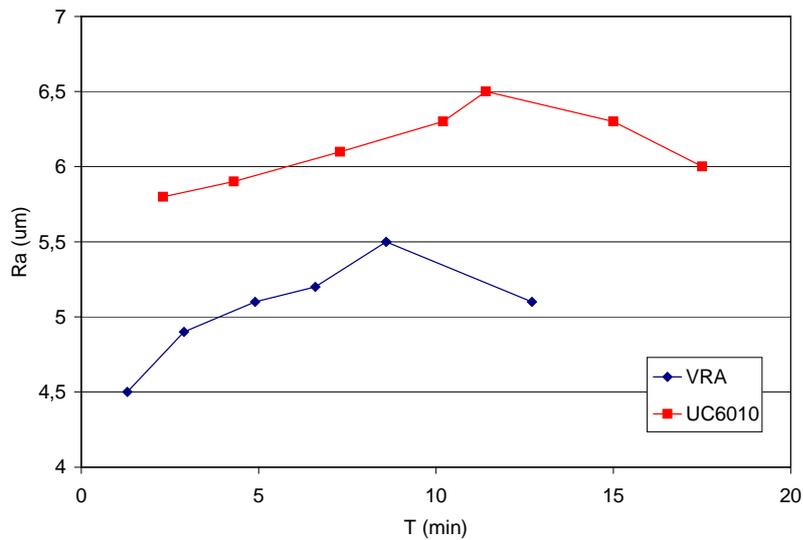
Figure 9. Average surface roughness (Ra) against cutting time for VRA and UC6010 tools ( $v_c=200$  m/min,  $f=0,4$  mm/rot e  $a_p=1$ mm).
