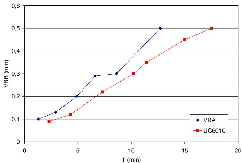
Figure 7. Tool wear against cutting time for VRA and UC6010 tools ( $v_c=200\text{ m/min}$ ,  $f=0,4\text{ mm/rot}$  e  $a_p=1\text{mm}$ ).
