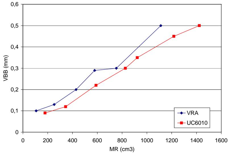
Figure 8. Tool wear against metal removal for VRA and UC6010 tools ( $v_c=200$  m/min,  $f=0,4$  mm/rot e  $a_p=1$ mm).
