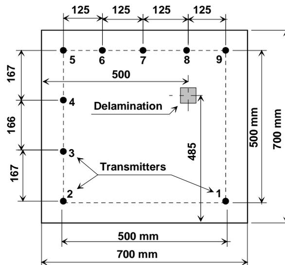
Figure 10: Experimental arrangement for acousto-ultrasonic detection
