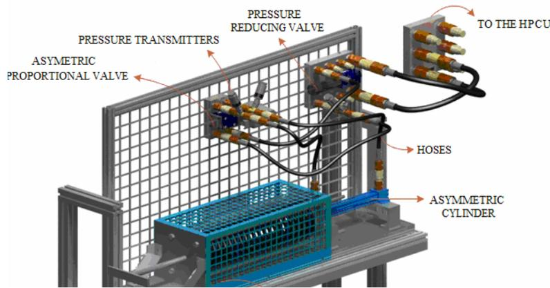
Figure 3. Workbench with a combination of asymmetric cylinder and asymmetric valve (SZPAK, 2008).
