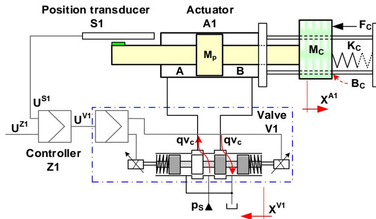
Figure 1. Electro-hydraulic system of positioning control (DE NEGRI, 2001).
