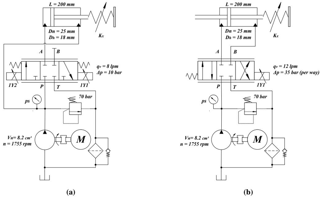
Figure 2. Electro-hydraulic circuits for positioning control: a) 3/3 AV+AC; b) 4/3 SV+SC.
