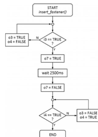
Figure 12. Insert fastener flowchart.
