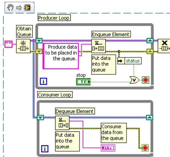
Figure 14. Producer/Consumer architecture example (National Instruments, 2013A).
