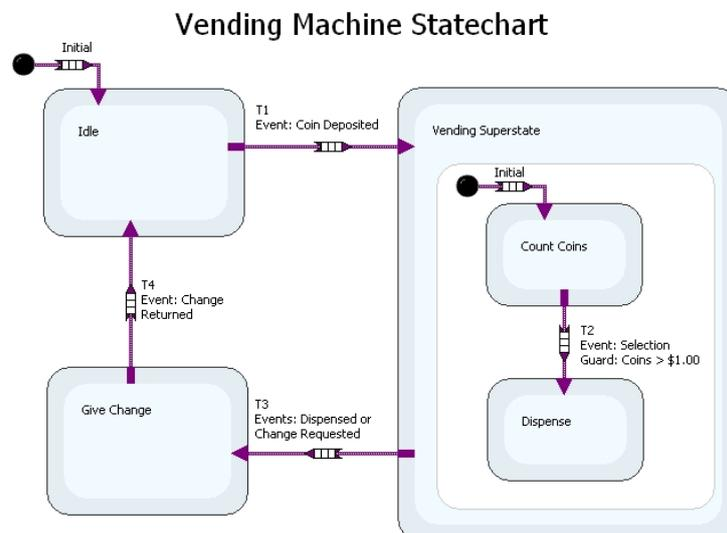
Figure 16. Statechart architecture example (National Instruments, 2013B).
