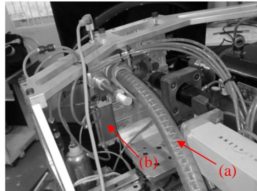
Figure 3. FARE and the hose for fasteners.
