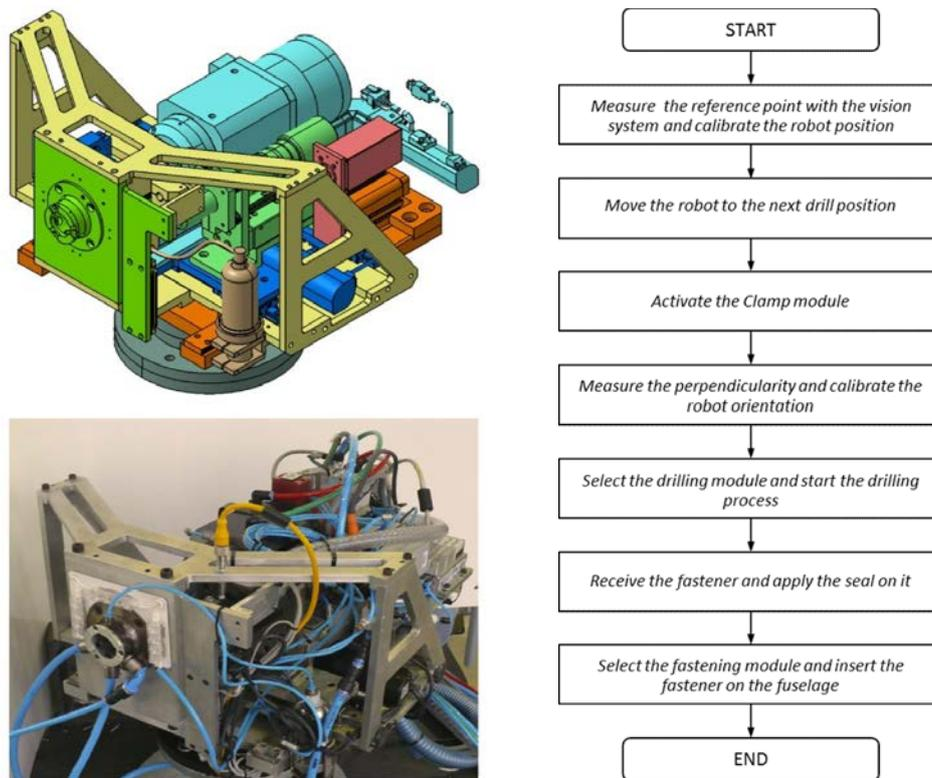
Figure 1. FARE (Fuselage Assembly Robotic end-Effector)
