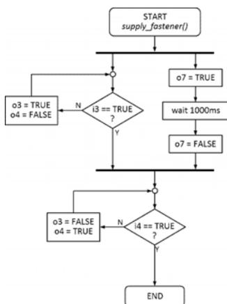
Figure 10. Supply the fastener on the inserter flowchart.
